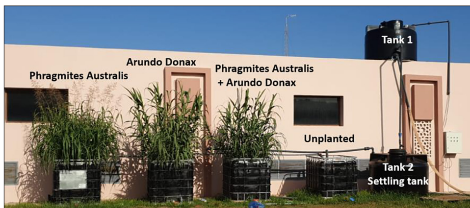
Figure 1. Overview of constructed wetland unit systems
