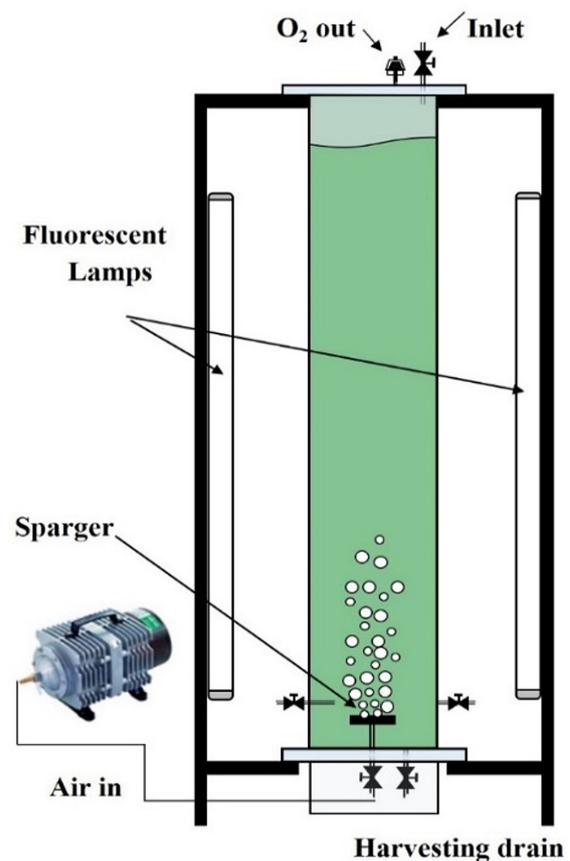
Figure 1. Schematic of FBR used in experimental work
