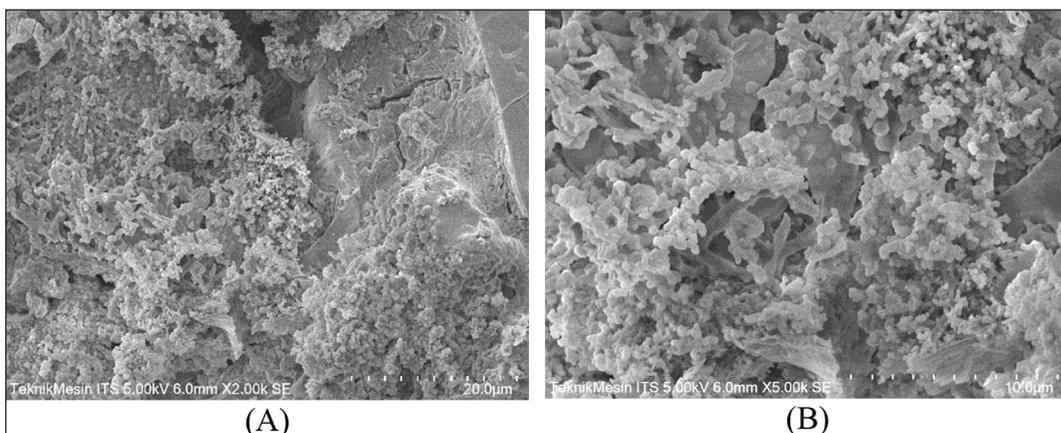
**Figure 10.** SEM micrograph of the precipitate. A)  $2.000\times$  magnification; B)  $5.000\times$  magnification
