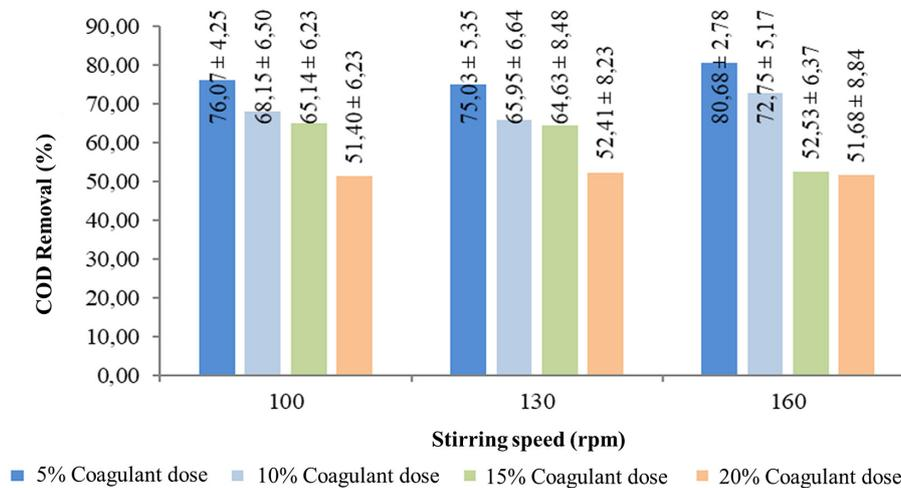
**Figure 4.** Average percentage reduction in COD concentration based on fast stirring speed (rpm)
