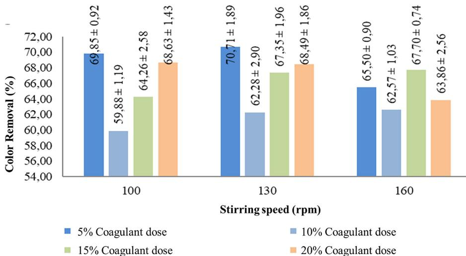
Figure 8. Average percentage decrease in dye absorbance based on rapid stirring speed (rpm)
