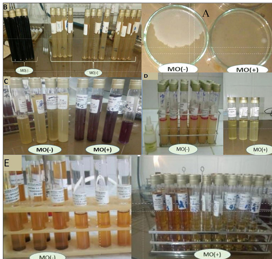
Figure 5. Demonstrations of some enumerations of total germs (A), sulfite-reducing Clostridium (B), total coliforms (C), fecal coliforms and E. coli (D), and total and fecal streptococci (E) in raw water. MO (+) presence of M. oleifera , MO (-) absence of M. oleifera
