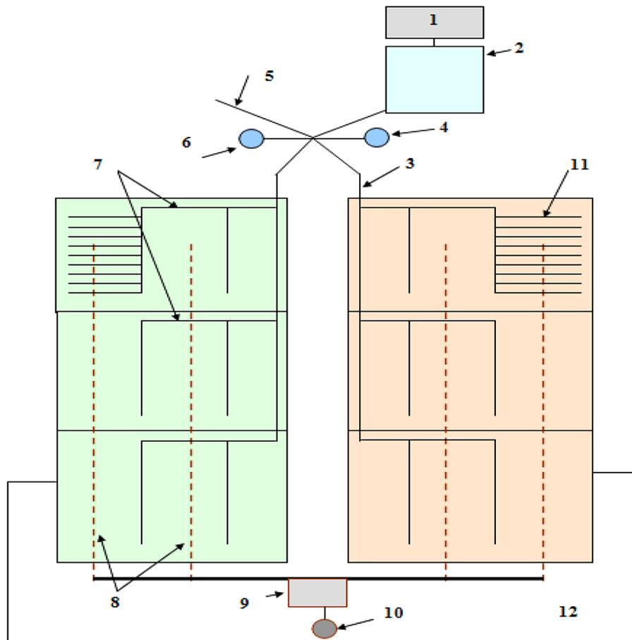
**Figure 1.** Schematic diagram of the irrigation system: 1 – wastewater treatment plants, 2 – storage pond, 3 – pumping station, 4 – distribution network for wastewater supply, 5 – distribution network for clean water supply, 6 – distribution hydraulic structure, 7 – precinct distribution channels, 8 – drainage network, 9 – the collector well, 10 – collector, 11 – temporary sprinklers, 12 – irrigation furrows
