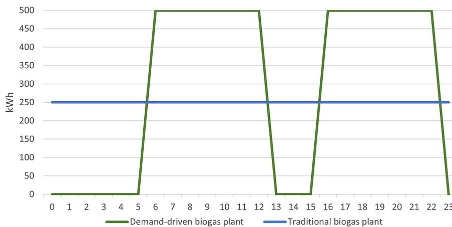
Figure 4. Comparison of the operation of a traditional biogas plant with demand-driven in the first variant
