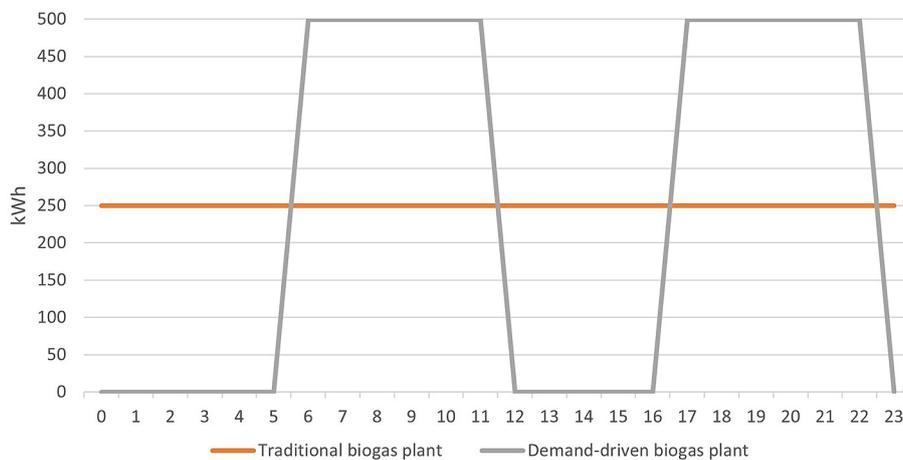
Figure 5. Comparison of the operation of a traditional biogas plant with demand-driven in the second variant
