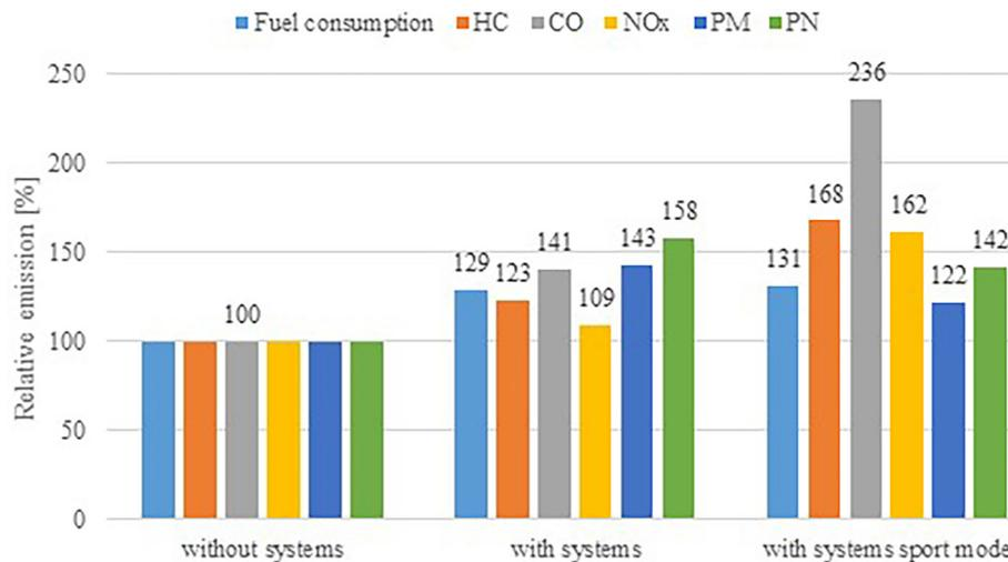
Figure 6. Vehicle 1 relative emissions in the WLTC cycle
