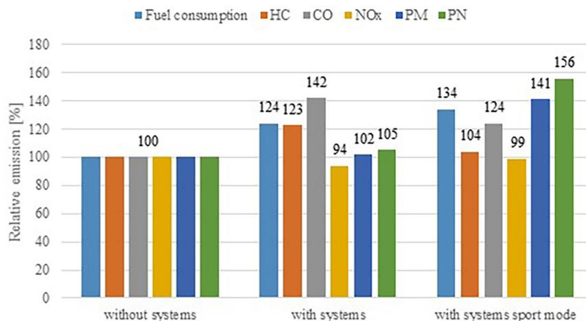
Figure 7. Vehicle 2 relative emissions in the WLTC cycle
