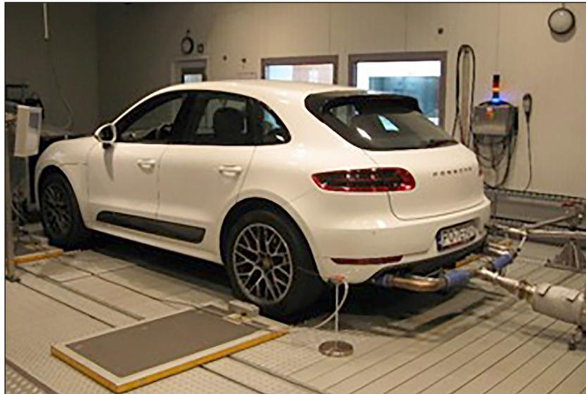
Figure 5. Exhaust gas uptake system during the test on the chassis dynamometer
