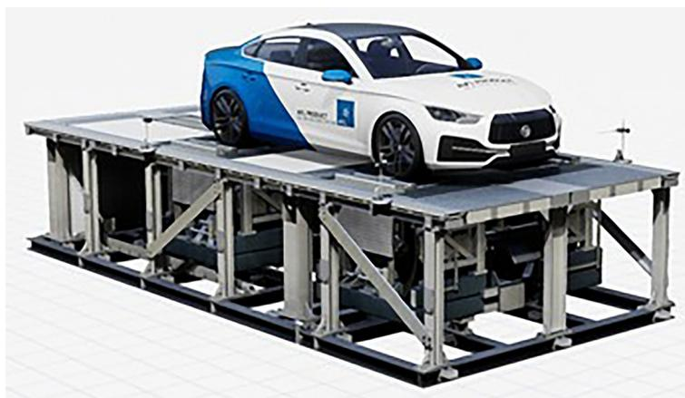
**Figure 3.** The equipment used for the measurements – AVL Dyno 48 4 × 4 chassis dynamometer
