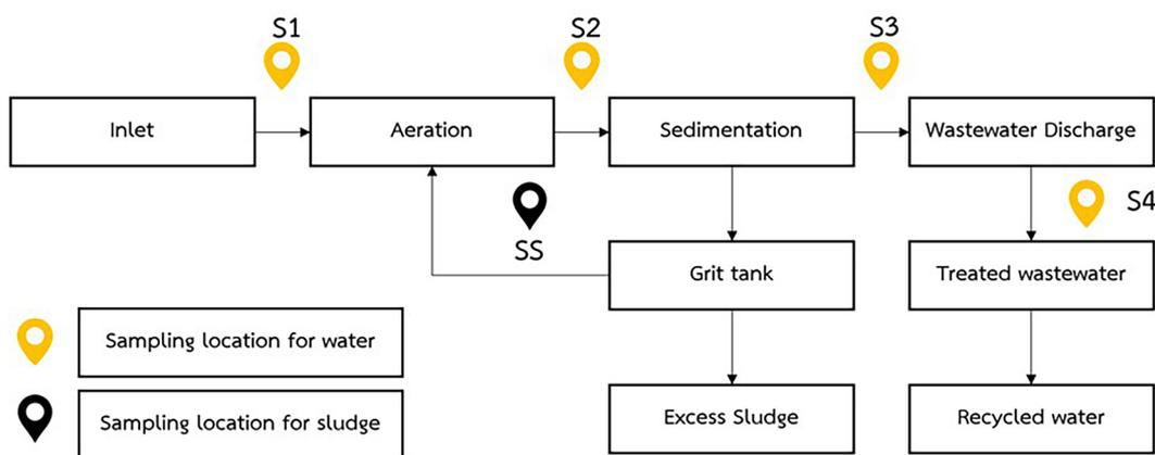
**Figure 1.** Schematic of the wastewater treatment system and sampling locations for wastewater and sediment
