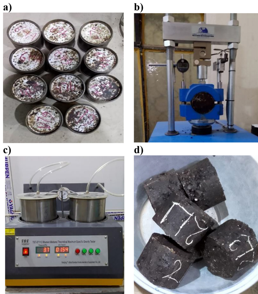
Figure 3. Marshall testing: (a) compacted sample, (b) Marshall device, (c) theoretical maximum specific gravity tester, (d) specimen fracture
