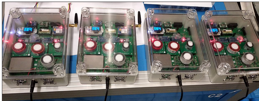
Figure 1. IAQmeters during tests after intercalibration
