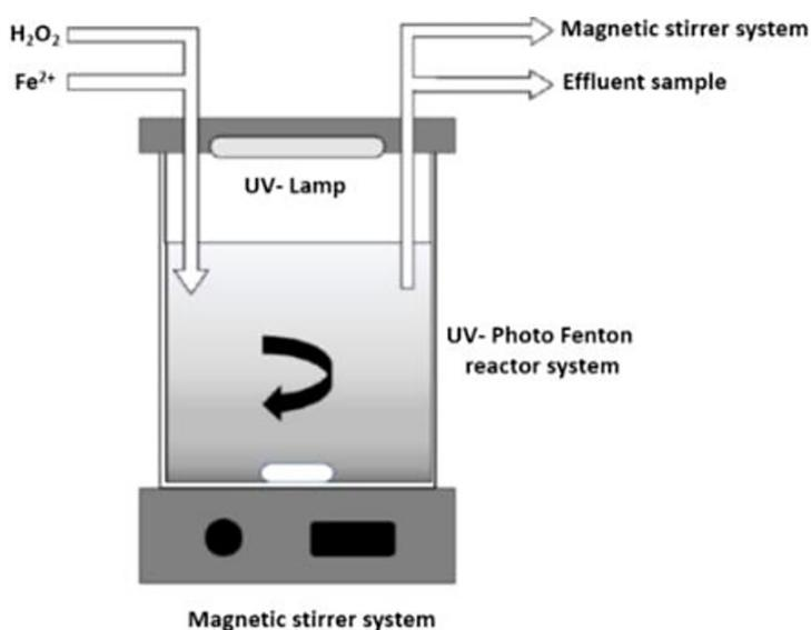
**Figure 1.** Schematic diagram of UV-photo-Fenton reactor
