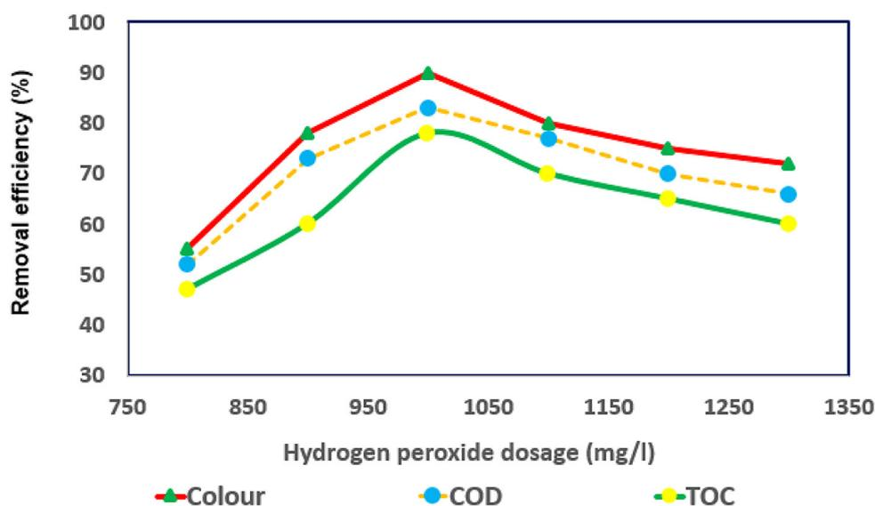
**Figure 4.** Effect of, hydrogen peroxide dose on pollutant removal efficiency at pH 4 with ferrous sulfate at 80 mg/l, and an irradiation time of 100 minutes
