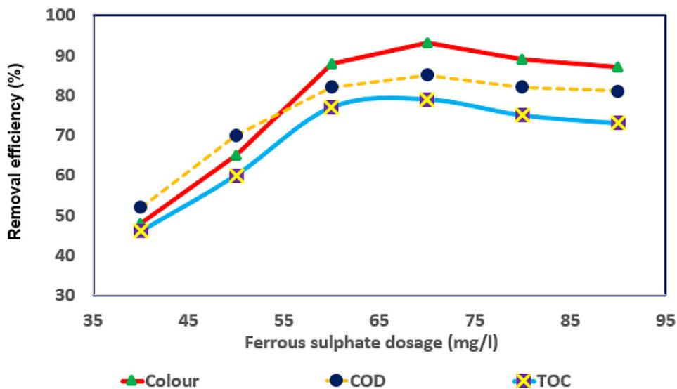
**Figure 5.** Effect of ferrous sulfate on the pollutant removal efficiency: pH 3, hydrogen peroxide of 900 mg/l, and irradiation time of 120 minutes
