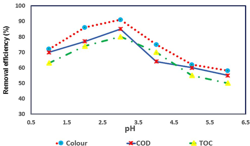
**Figure 2.** Effect of pH on the pollutant removal efficiency: Irradiation time of 80 minutes, hydrogen peroxide of 900 mg/l, and ferrous sulfate of 60 mg/l
