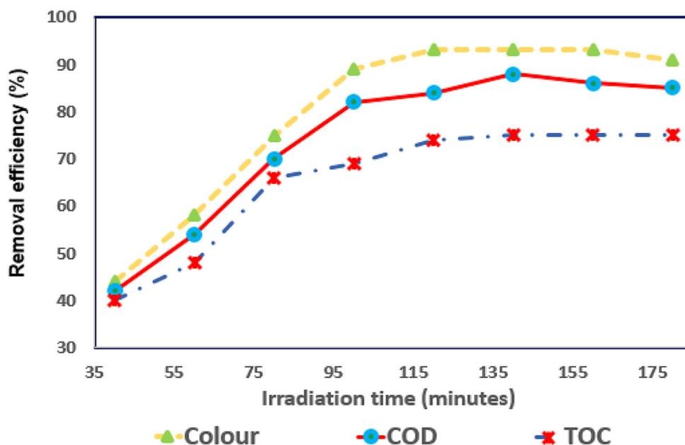
**Figure 3.** Effect of irradiation time on the pollutant removal efficiency: pH 3, hydrogen peroxide of 800 mg/l, and ferrous sulfate of 70 mg/l
