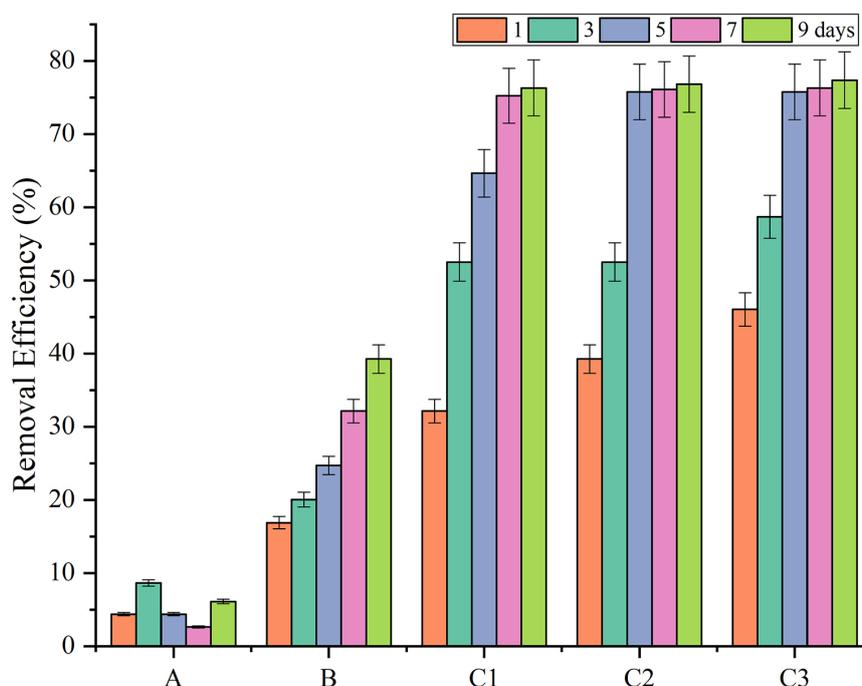
**Figure 4.** The effect of detention time on COD removal efficiency. The different treatments were A (control POME only), B (control POME and plant), C1 (POME, plant and polymer, polymer ratio: 0.5), C2 (POME, plant and polymer, polymer ratio: 0.4), C3 (POME, plant and polymer, polymer ratio: 0.3)
