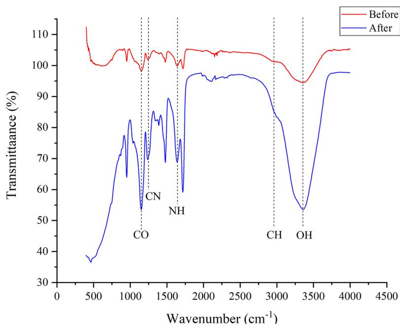
**Figure 6.** Fourier transform infrared (FTIR) of polymer before and after treatment (C3)
