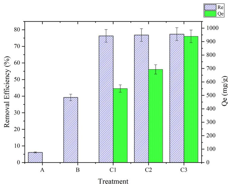
**Figure 2.** The effect amount of polymer on COD removal efficiency and adsorption capacity. The different treatments were A (control POME only), B (control POME and plant), C1 (POME, plant and polymer, polymer ratio: 0.5), C2 (POME, plant and polymer, polymer ratio: 0.4), C3 (POME, plant and polymer, polymer ratio: 0.3), Qe means adsorption capacity
