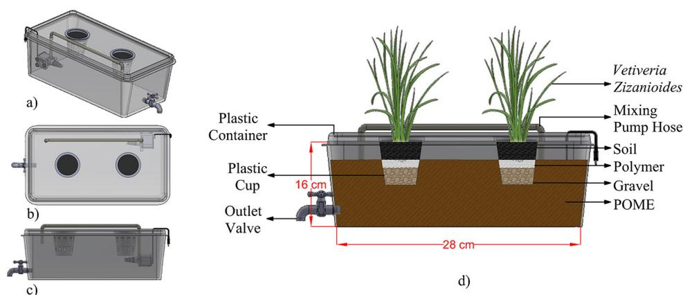
**Figure 1.** Reactor configuration at: (a) 3D view, (b) top view, (c) side view, (d) experimental setup
