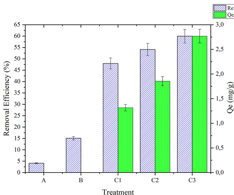
**Figure 3.** The effect amount of polymer on phosphate removal efficiency and adsorption capacity. The different treatments were A (control POME only), B (control POME and plant), C1 (POME, plant and polymer, polymer ratio: 0.5), C2 (POME, plant and polymer, polymer ratio: 0.4), C3 (POME, plant and polymer, polymer ratio: 0.3), Qe means adsorption capacity
