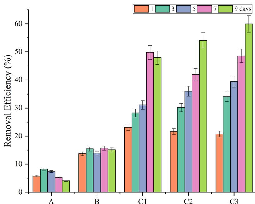
**Figure 5.** The effect of detention time on phosphate removal efficiency. The different treatments were A (control POME only), B (control POME and plant), C1 (POME, plant and polymer, polymer ratio: 0.5), C2 (POME, plant and polymer, polymer ratio: 0.4), C3 (POME, plant and polymer, polymer ratio: 0.3)
