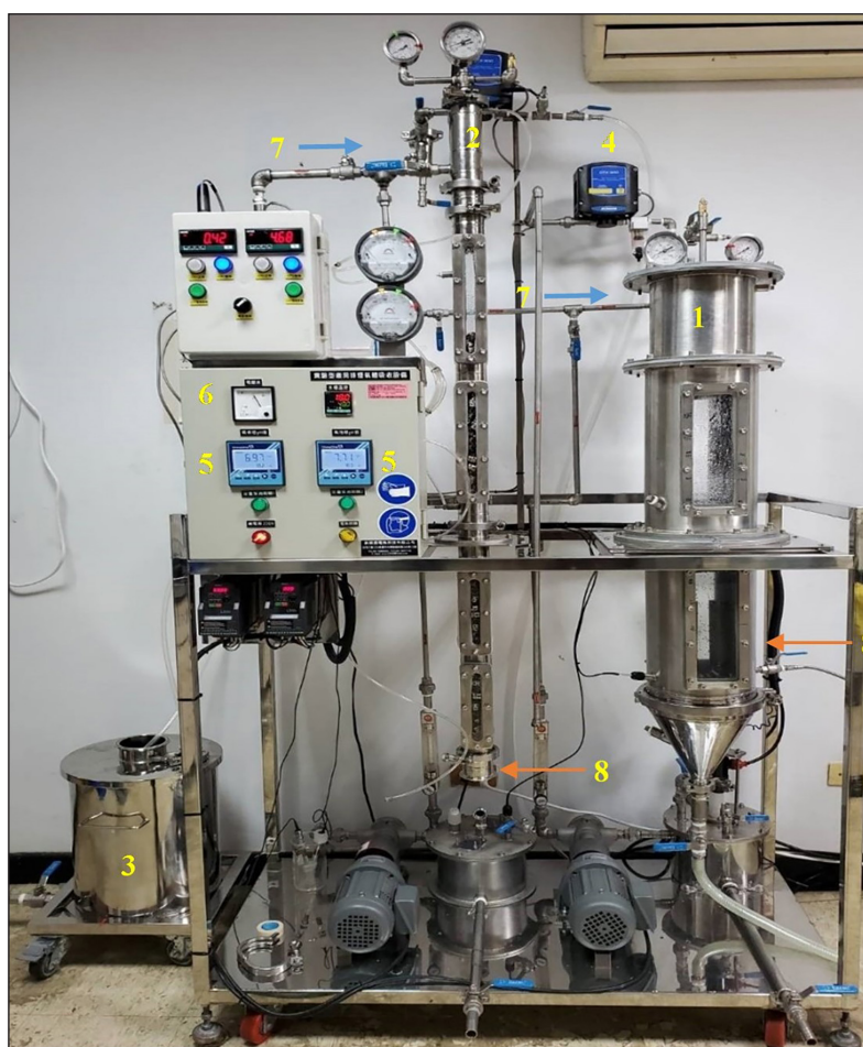
Figure 1. Photo of bench-scale experiments for CO 2 captured and mineral carbonation in NaOH. solution: 1 –bubble column reactor, 2 – packed bed reactor, 3 – NaOH solution tank, 4 – CO 2 analyzer, 5 – pH meter, 6 –instrument indicator, 7 – absorbent inlet flow, 8 – CO 2 inlet flow
