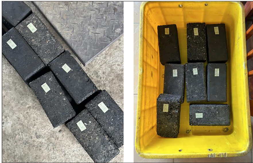
Figure 1. Paving block made from non-economic plastic waste and aggregate
