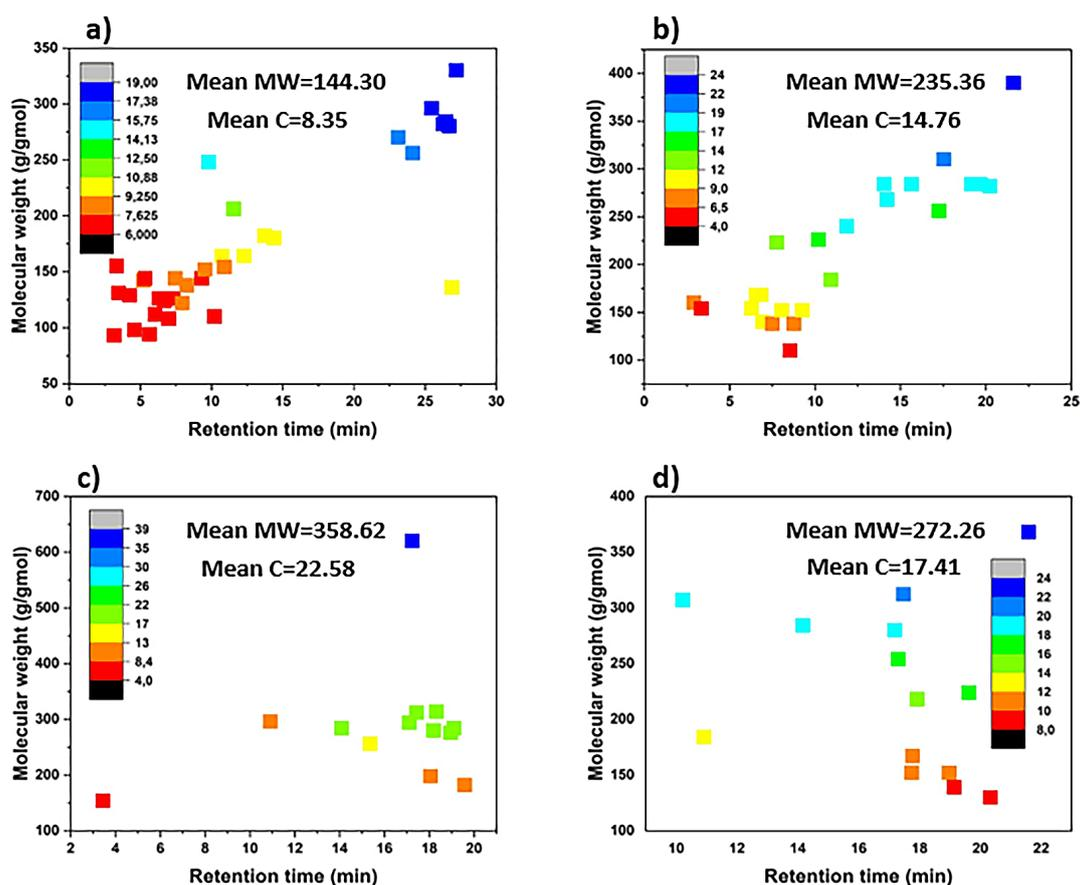
Figure 11. Carbon distribution of rice husk pyrolysis product in (a) water phase (liquid smoke) at 400 °C, (b) tar at 400 °C, (c) tar at 500 °C, (d) tar at 600 °C
