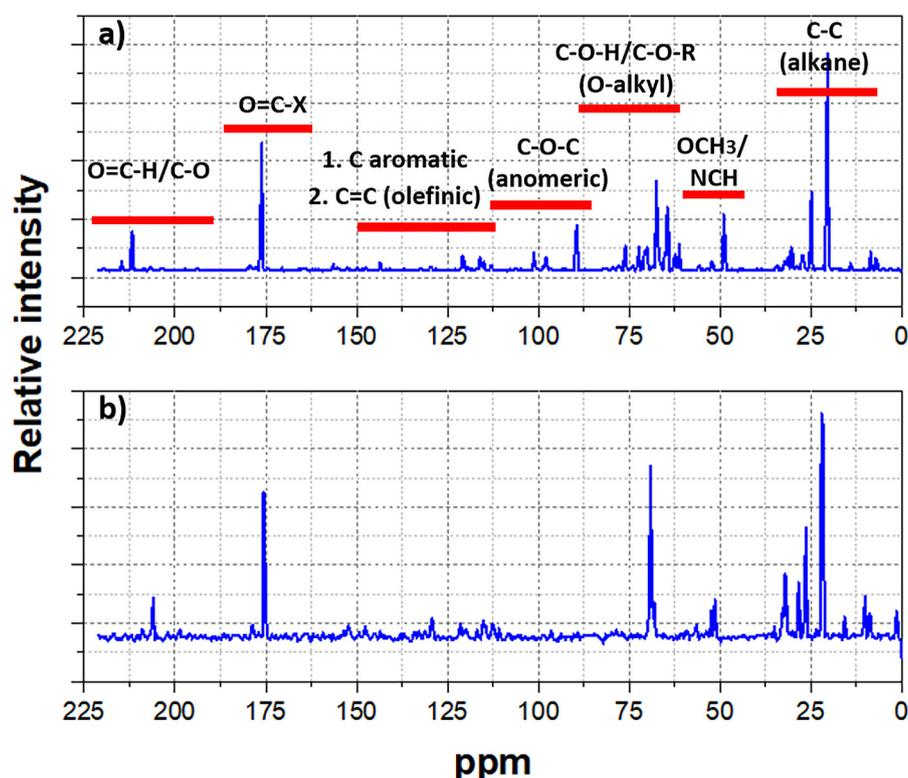
**Figure 3.** <sup>13</sup>C-NMR spectra of rice husk pyrolysis product: (a) water phase (liquid smoke) product at 400 °C, (b) tar product at 400 °C
