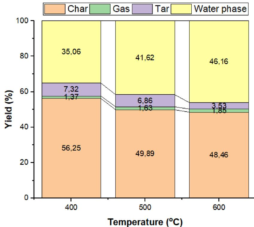
Figure 5. The yield of pyrolysis product at different pyrolysis temperatures
