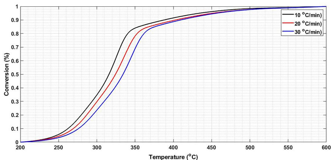
Figure 2. Thermogravimetry analysis (TGA) curve of rice husk decomposition
