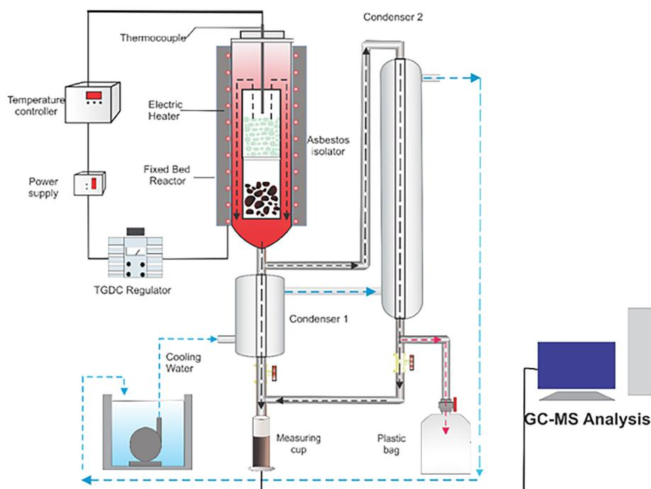
**Figure 1.** Experimental setup of rice husk pyrolysis
