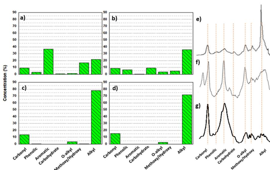
**Figure 9.** Carbon species distribution of (a) water phase (liquid smoke) at 400 °C, (b) tar at 400 °C, (c) tar at 500 °C, (d) tar at 600 °C, (e) humin of Muck Crops soil, (f) fulvic acid cow manure, (g) humic acid of IHSS Mollisol standard soil
