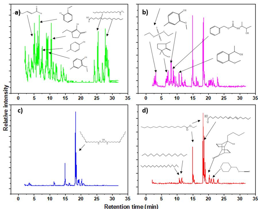
Figure 6. GC-MS spectra of pyrolysis product (a) water phase (liquid smoke) at 400 °C, (b) tar 400 °C, (c) tar 500 °C, (d) tar 600 °C
