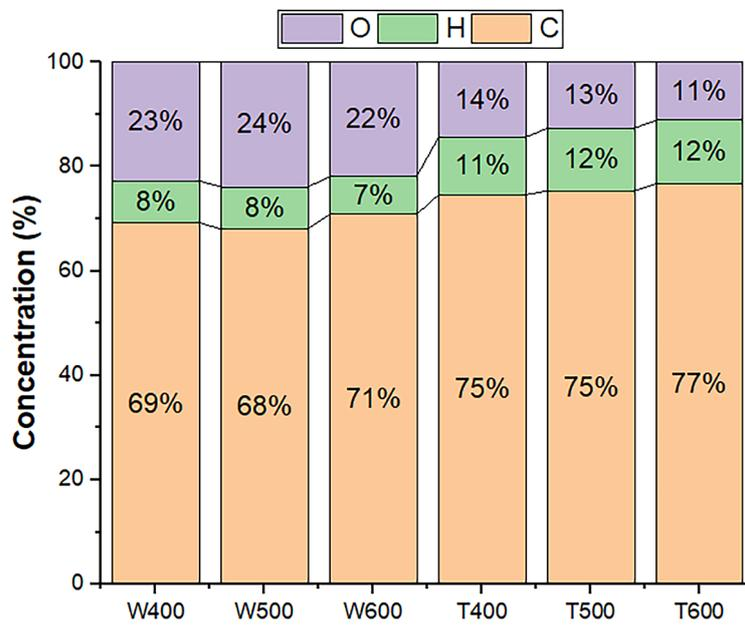
Figure 12. Carbon, hydrogen, and oxygen content in the liquid product of pyrolysis
