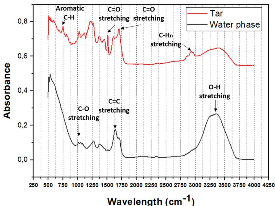
**Figure 4.** FT-IR spectra of water phase (liquid smoke) and tar product of rice husk pyrolysis
