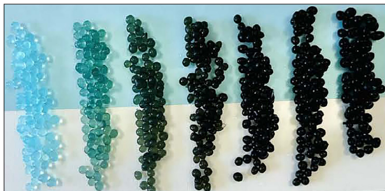
Figure 11. Photo of the granules after methyl blue sorption on pure alginate granules (A0 – first on the left) and composite granules (A1 – A6, second and subsequent from the left)
