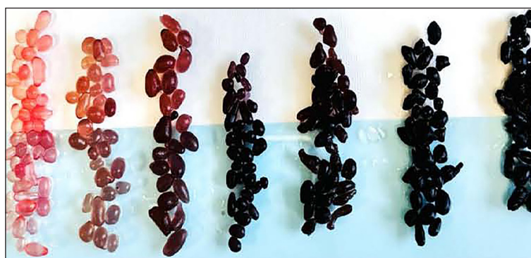
Figure 13. Photo of the granules after Congo red sorption on pure alginate granules (A0 – first on the left) and composite granules (A1–A6, second and subsequent from the left)
