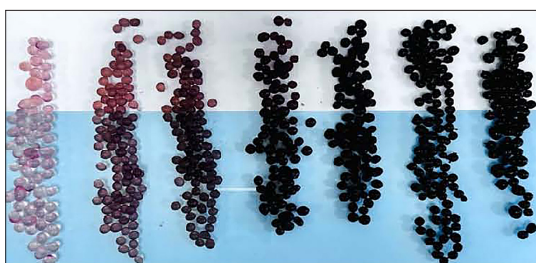
Figure 15. Photo of the granules after orange II sorption on pure alginate granules (A0 – first on the left) and composite granules (A1–A6, second and subsequent from the left)
