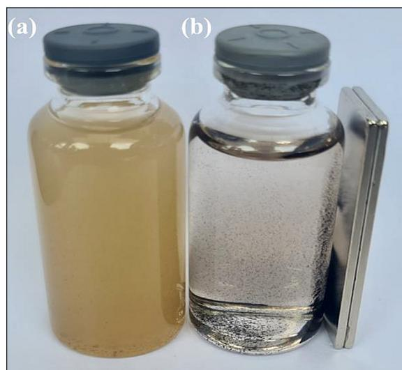
**Figure 7.** Raw water before and after treatment using activated carbon/ $\text{NiFe}_2\text{O}_4$  composite
