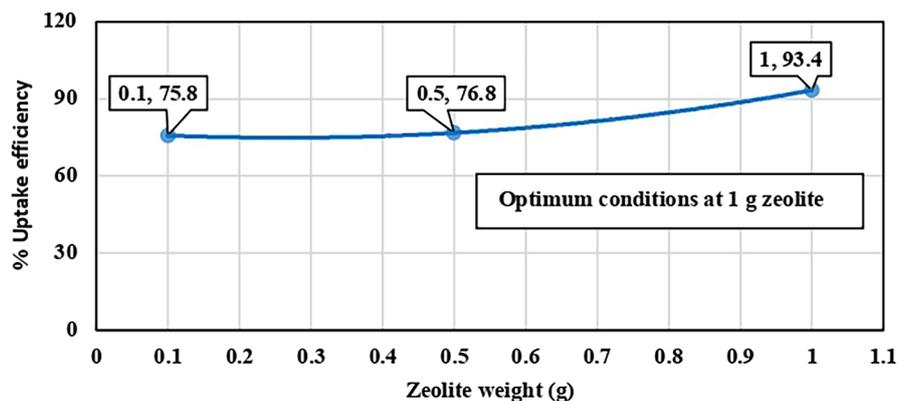
**Figure 3.** The uptake efficiency of SDBS-MBAS at (0.1, 0.5, 1.0) g at Ph = 6.8 and time 30 minute
