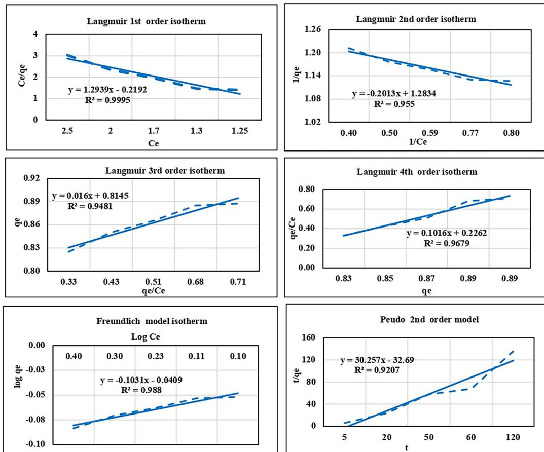
**Figure 4.** The adsorption isotherms of SDBS-MBAS with liner equations and coefficient of determination  $R^2$
