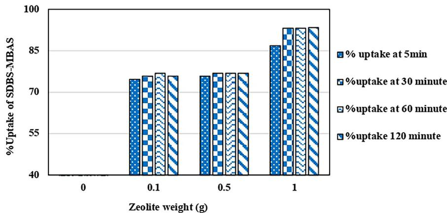
**Figure 1.** The uptake efficiency of SDBS-MBAS surfactant at (0.1, 0.5, 1.0) g of zeolite at different mixing time durations
