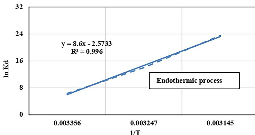
**Figure 2.** The relationship between the partition adsorption coefficient ( $K_d$  in L/g) of SBDS-MBAS at 1 g zeolite and pH=6.8 at different temperatures in Kelvin as (298, 308, and 318)
