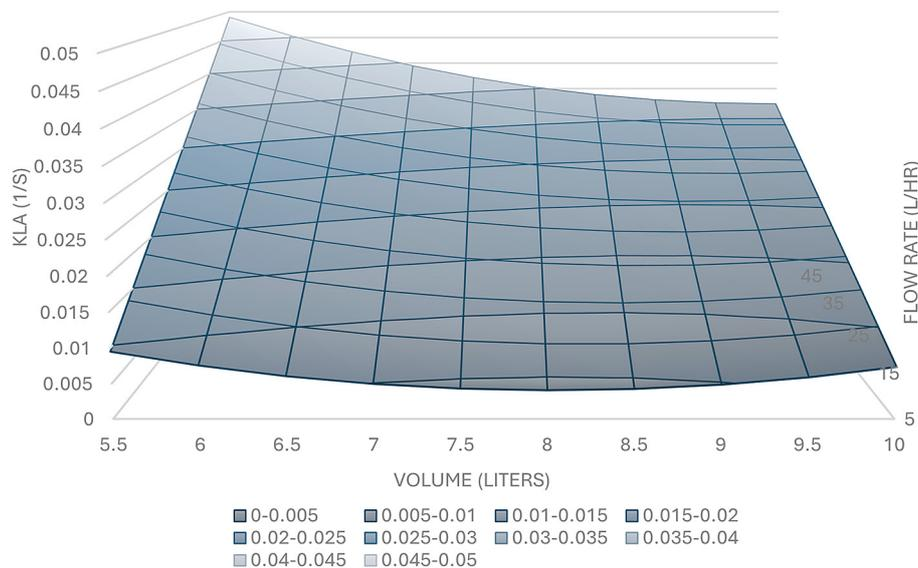
Figure 6. Surface plot for KLa vs flow rate and volume
