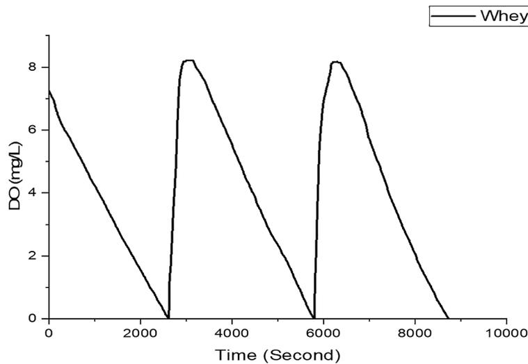
Figure 8. Figure showing the dissolution of oxygen in a solution and the organism’s consumption of oxygen at a flow rate of 50 L/h
