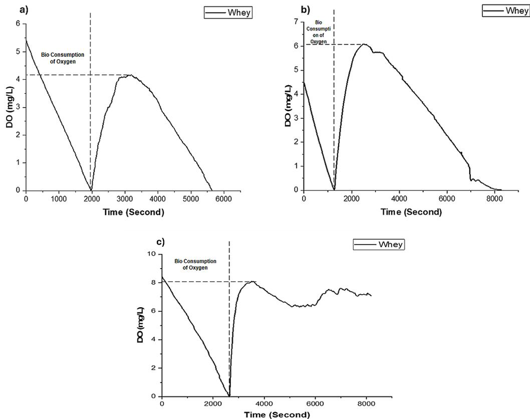
**Figure 9.** Organism's consumption of oxygen at a flow rate: a) 5 L/h, b) 15 L/h, c) 25 L/h
