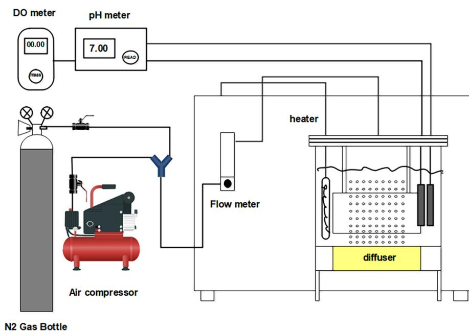
Figure 1. Schematic diagram of the airlift bioreactor experimental setup
