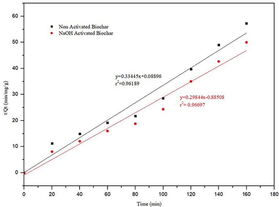
**Figure 9.** Pattern of PSO adsorption kinetic pattern for Remazol yellow onto coffee fruit shell biochar adsorbent
