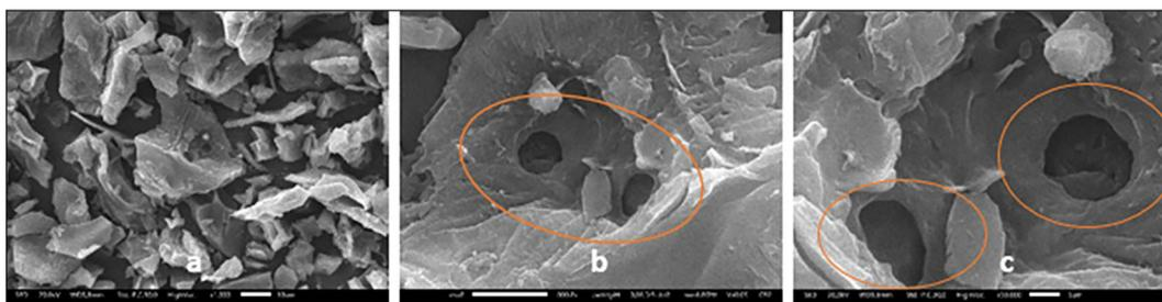
**Figure 2.** Morphological analysis of NaOH-activated biochar at ((a) 1000× magnification, (b) 5000× magnification, (c) 10,000× magnification)
