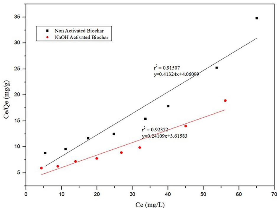
Figure 6. Langmuir adsorption isotherm pattern on coffee fruit shell biochar
