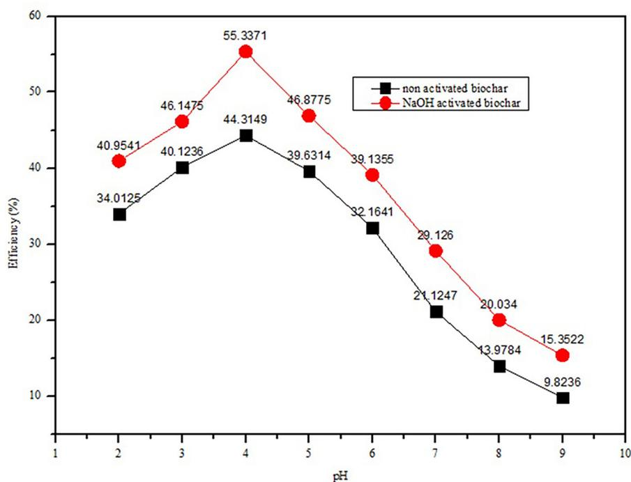
**Figure 3.** The relationship between pH variation and adsorption efficiency
