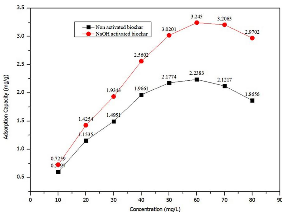
Figure 5. Graph of the relationship between the initial concentration of Remazol yellow FG dye by coffee fruit shell biochar and the adsorption capacity
