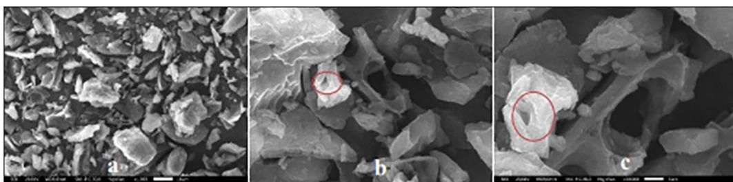
**Figure 1.** Morphological analysis of nonactivated biochar at ((a) 1.000× magnification, (b) 5.000× magnification, (c) 10.000× magnification)
