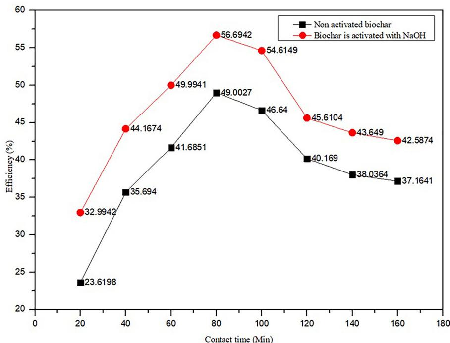
**Figure 4.** The relationship graph between contact time variation (minutes) and efficiency
