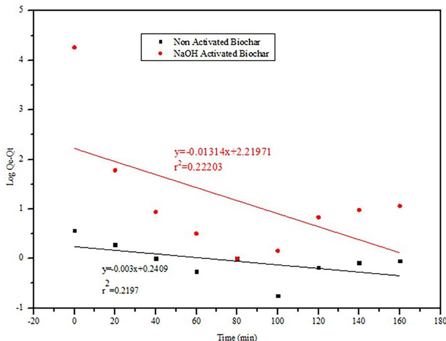
Figure 8. Pattern of PFO adsorption kinetic for Remazol yellow onto the coffee fruit shell biochar adsorbent
