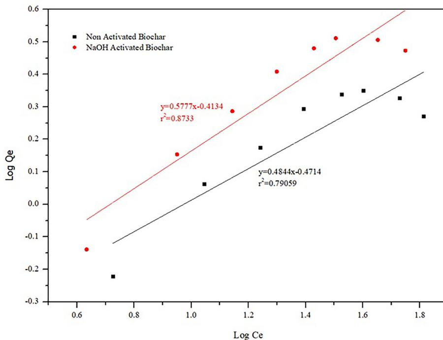
Figure 7. Freundlich adsorption isotherm pattern on coffee fruit shell biochar adsorbent
