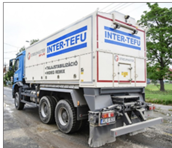
Figure 1. Mercedes truck equipped with a delivery and spreader system
