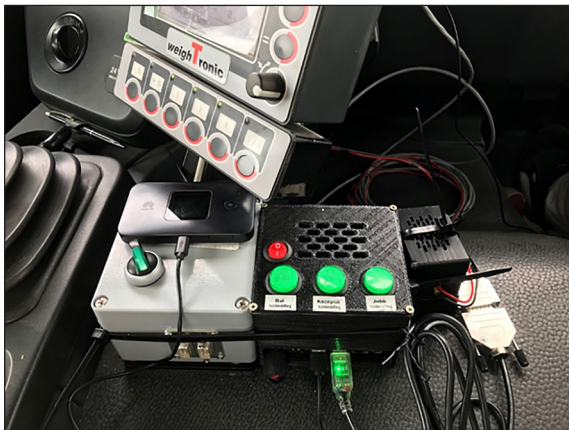
Figure 3. Placement of the system's control unit in the vehicle's cabin
