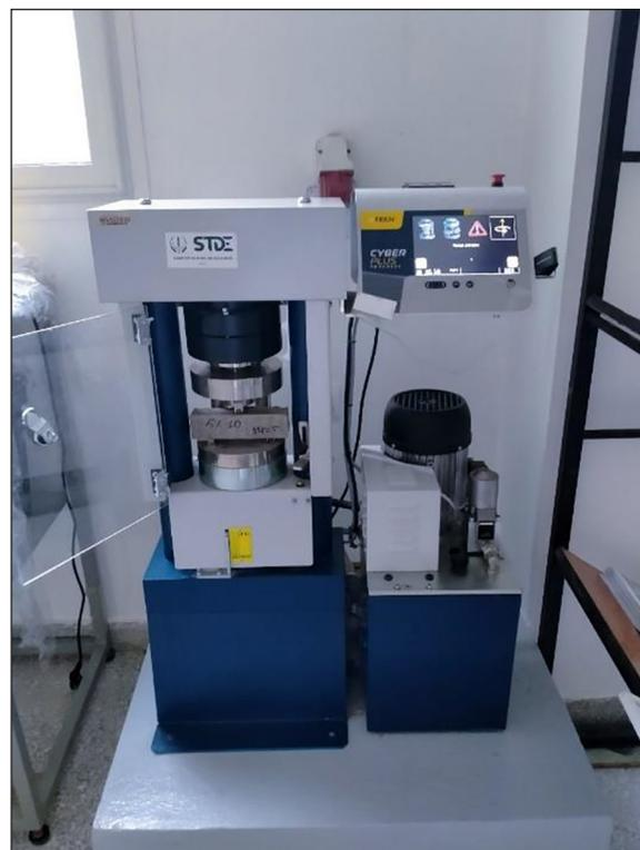
**Figure 3.** Compression press used for testing schist-based mortar samples
