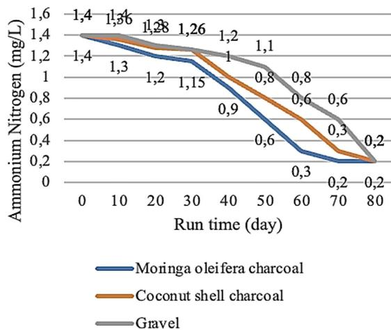
Figure 8. Ammonium removal in bio SSF
