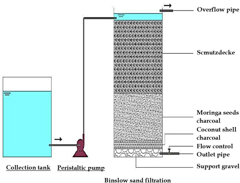
Figure 1. Schematic diagram of bio-slow sand filtration
