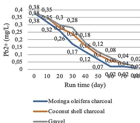
Figure 6. Pb<sup>2+</sup> removal in bio SSF
