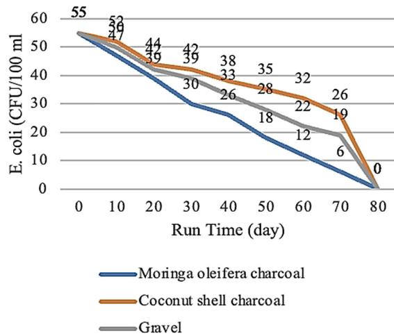
Figure 3. E. coli removal in bio SSF
