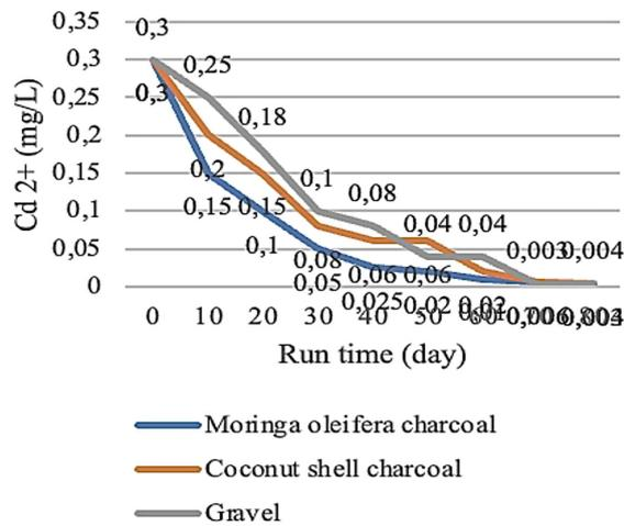
Figure 7. Cd<sup>2+</sup> removal in bio SSF
