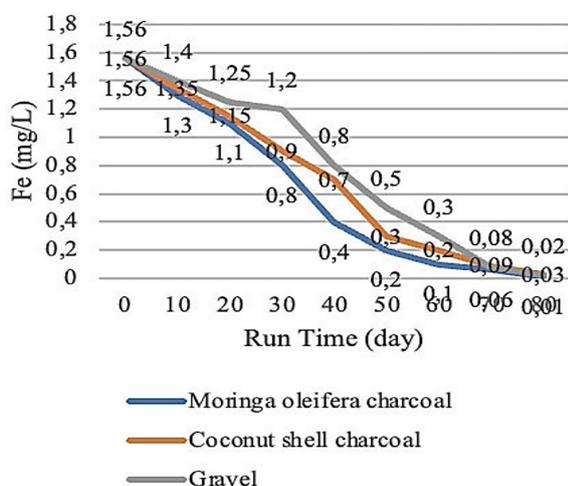
Figure 5. Fe removal in bio SSF
