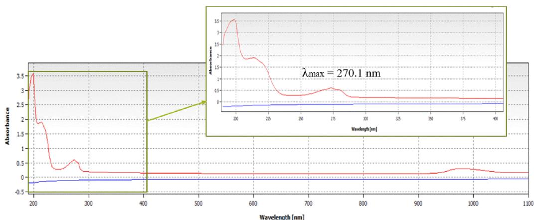
Figure 2. Absorption curve for phenol with concentration of 25 ppm
