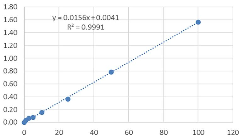
**Figure 3.** Calibration curve of phenol by using UV-VIS technique
