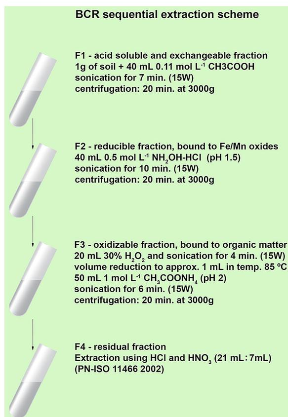
**Figure 1.** The ultrasound accelerated sequential extraction procedure for metal fractionation according to BCR (Community Bureau of Reference)
