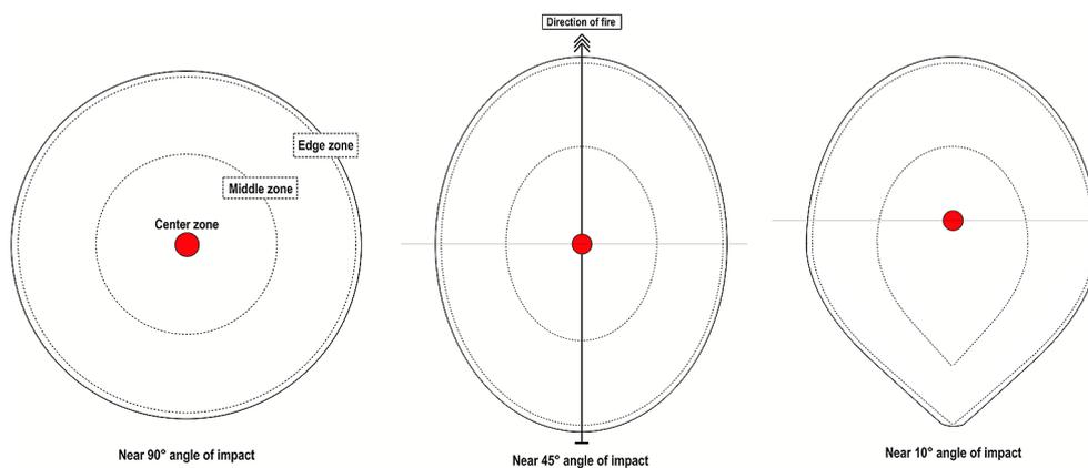
**Figure 5.** Shell crater shapes according to angles of impact
