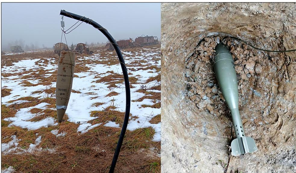
**Figure 1.** Static initiation of 152 mm artillery shell and 120 mm mortar bomb
