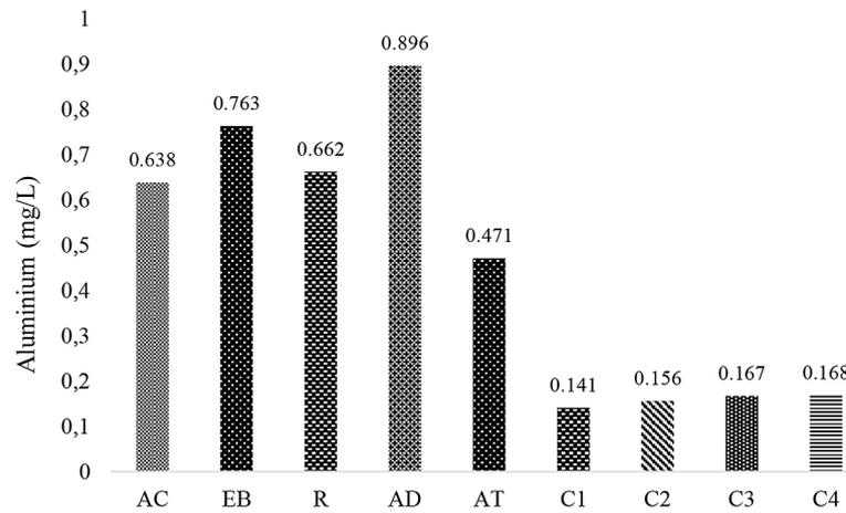
**Figure 6.** The concentration of aluminum in water. AC (raw water), EB (reservoir), R (river), AD (decantation water), AT (treated water), C (houses)
