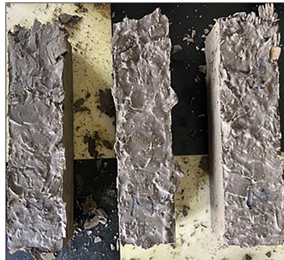
Figure 3. Texture of sample with chips after deformation (photo by A. Krajewska)
