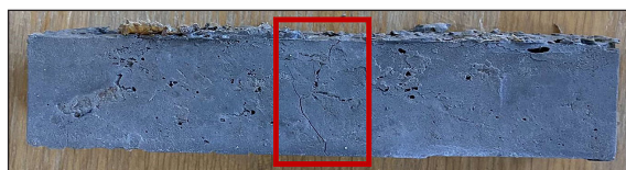
Figure 4. Scratching of a beam with a large chip fraction after exceeding the bending strength (photo by A. Krajewska)
