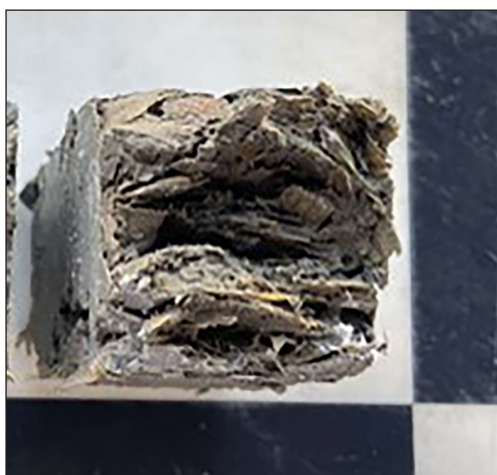
Figure 5. Section of a beam with a large chip fraction (photo by A. Krajewska)
