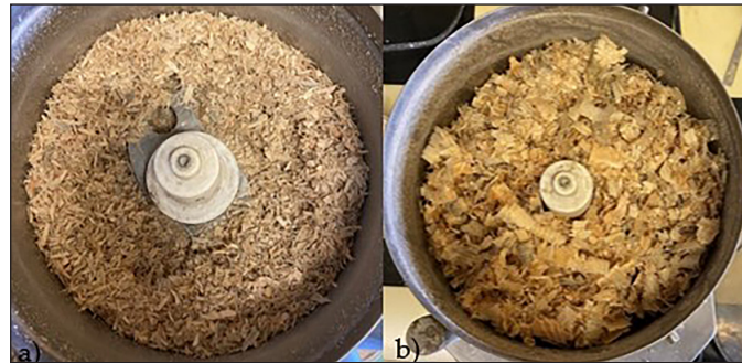
Figure 8. Fraction of chips a) after blend, fine fraction b) before blend, thick fraction (photo by A. Krajewska)
