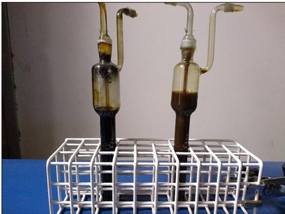
Figure 11. Impinger bottles with the isopropanol-liquid fraction solution
