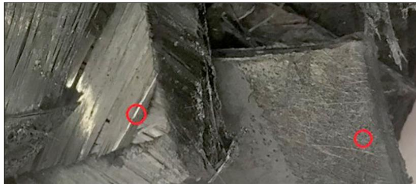
**Figure 4.** Photography of pyrolyzed samples: straight fiber composite (left) and disordered fiber composite with heavy hydrocarbons present on the surface (right). Red marks refer to Figure 5 and Figure 6.
