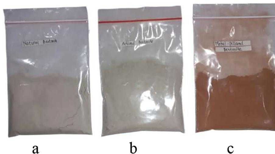
**Figure 1.** Catalyst materials: (a) natural bentonite, (b) activated bentonite, and (c) metal-pillared bentonite
