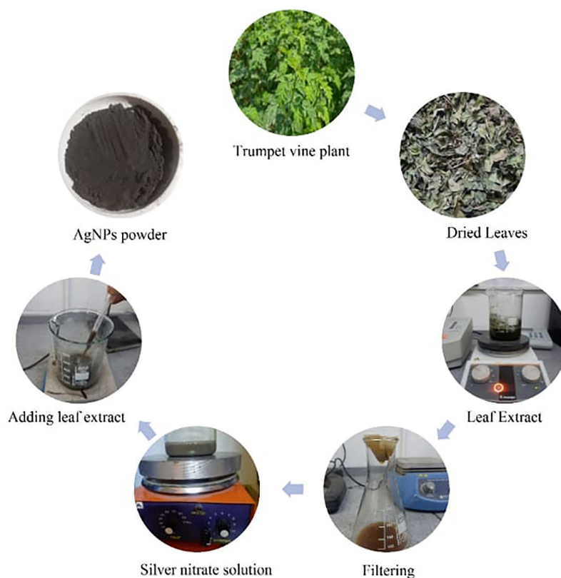
Figure 1. Flowchart illustrates the green synthesis process of Ag 2 O nanoparticles
