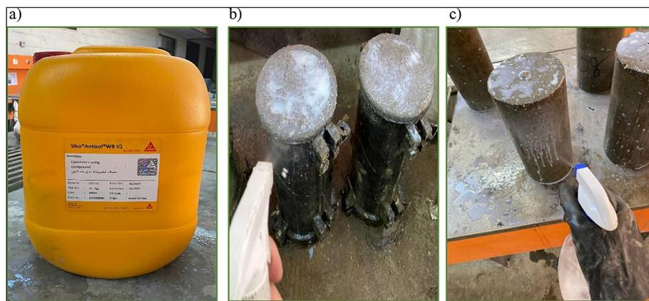
**Figure 8.** Liquid membrane-forming compound: (a) Sika Antisol WB, (b) after initial moist, (c) after removal from the mold
