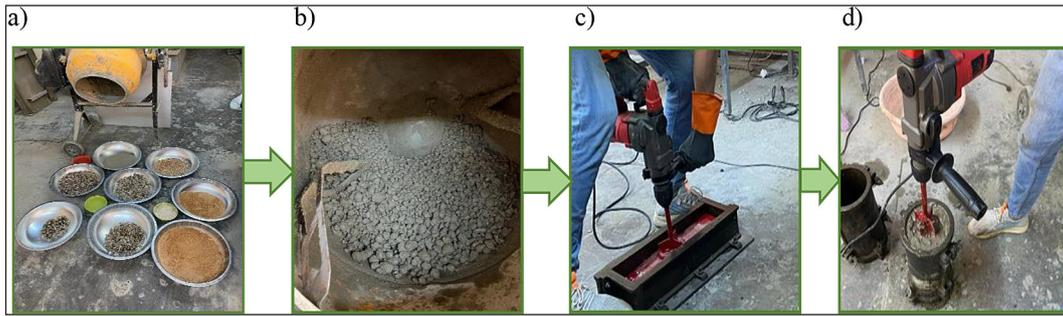
**Figure 6.** Compacting procedures according to ASTM C1435: (a) preparing ingredients, (b) ingredients after mixing, (c) compaction technique for cylinder, (d) compaction technique for prism
