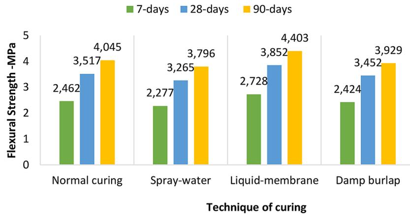
Figure 14. The results of flexural-strength test with different curing techniques
