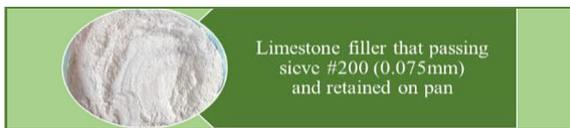
Figure 3. Crushed-limestone aggregate
