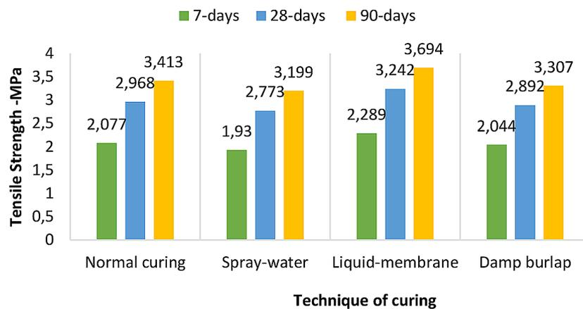
Figure 12. The results of tensile strength test with different curing techniques
