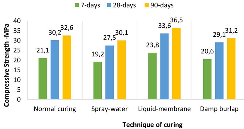
**Figure 10.** The results of compressive-strength test with different curing techniques
