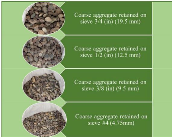
Figure 1. Utilized coarse-aggregate
