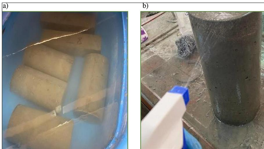
**Figure 7.** Curing of samples: (a) normal curing, (b) spray-water curing
