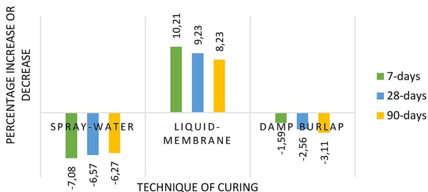
Figure 13. The percentage of tensile strength test compared with normal curing
