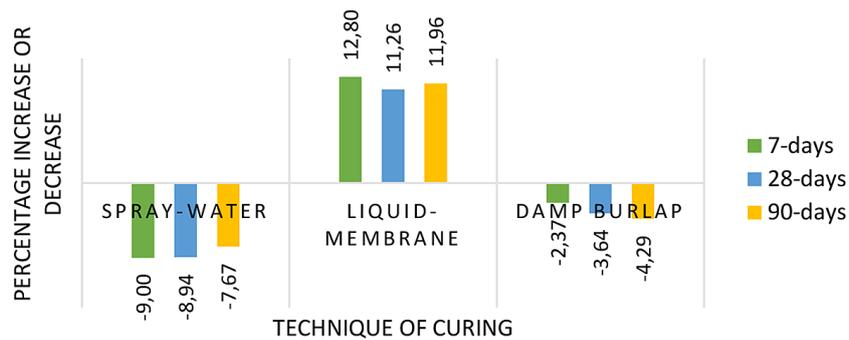
**Figure 11.** The percentage of compressive-strength test compared with normal curing
