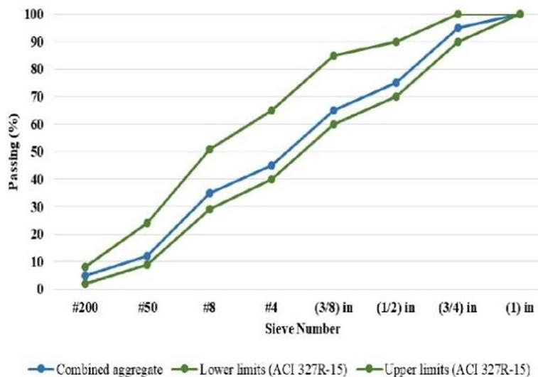
Figure 4. Combined-aggregate-gradation
