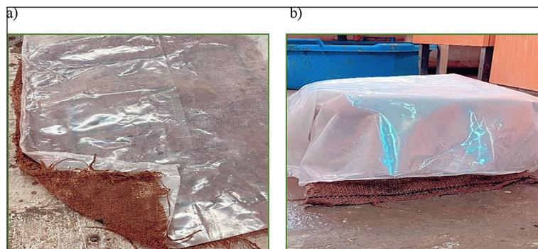
**Figure 9.** Damp burlap curing: (a) burlap-white-polyethylene-sheet, (b) after casing
