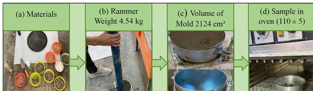
**Figure 5.** Modified proctor test steps according to ASTM D1557: (a) Preparing materials and mixing, (b) Tamping the specimen, (c) weight the mold, (d) The specimen in oven
