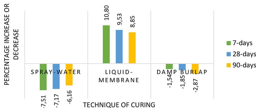
Figure 15. The percentage of flexural-strength test compared with normal curing
