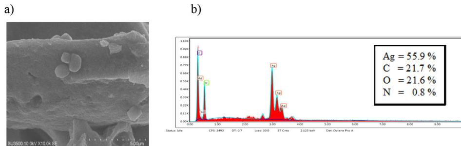
**Figure 3.** Electron microscopy study: (a) SEM analysis and (b) Energy-dispersive x-ray (EDX) Spectra of AgNPs
