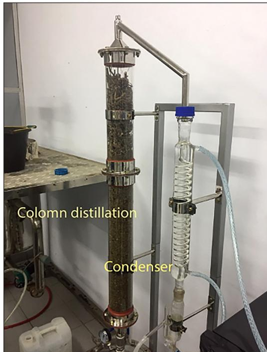
**Figure 2.** Photograph of the experimental setup
