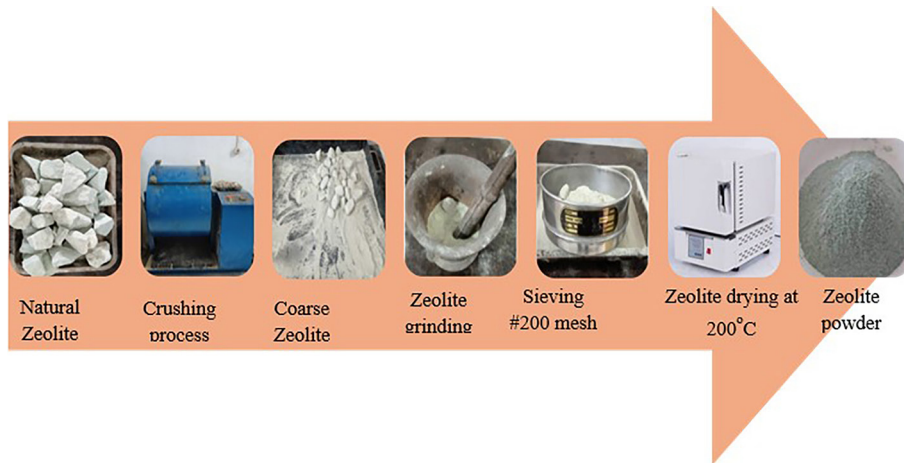
Figure 2. Preparation process of zeolite from natural form to powder
