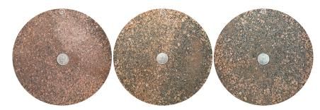
Figure 6. Lime mortar mixture compositions: (a) M1, (b) M2, (c) M3
