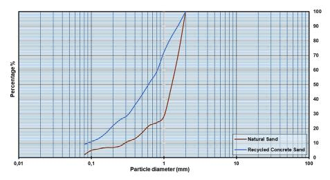
Figure 9. Particle size distribution of natural sand and recycled concrete sand
