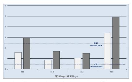
Figure 11. Compressive strengths of mortar mixes at different ages
