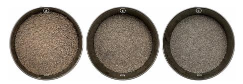
Figure 3. Varieties of sands employed in mortar mixtures; (a) raw natural sand, (b) washed natural sand, (c) recycled concrete sand
