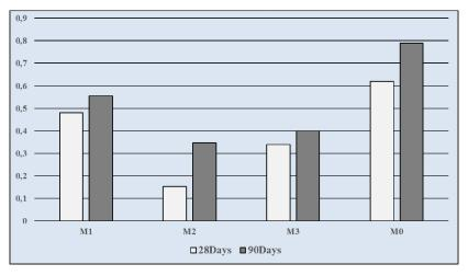
Figure 12. Flexural strengths of mortar mixes at different ages
