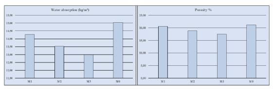
Figure 13. Water absorption and porosity results of mortar mixes at different ages
