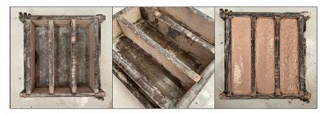
Figure 8. Prism specimens for mortar mix testing
