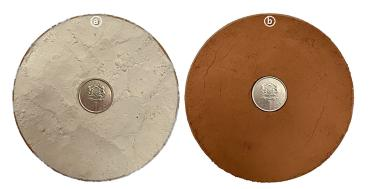
Figure 4. Varieties of binders employed in mortar mixtures; (a) aerial lime, (b) recycled brick powder
