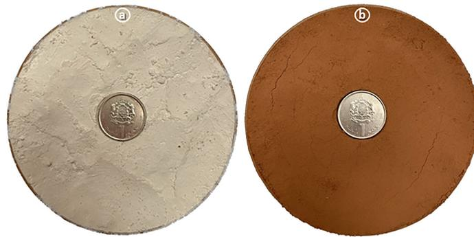
Figure 4. Varieties of binders employed in mortar mixtures; (a) aerial lime, (b) recycled brick powder
