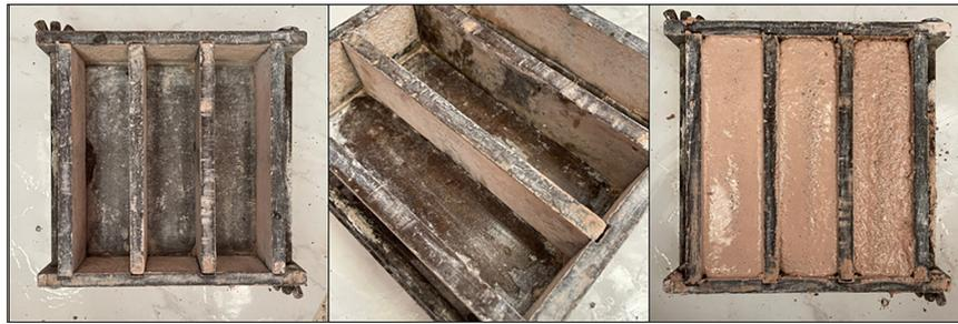
Figure 8. Prism specimens for mortar mix testing
