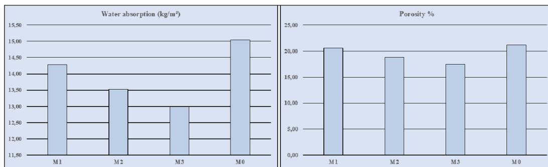
Figure 13. Water absorption and porosity results of mortar mixes at different ages
