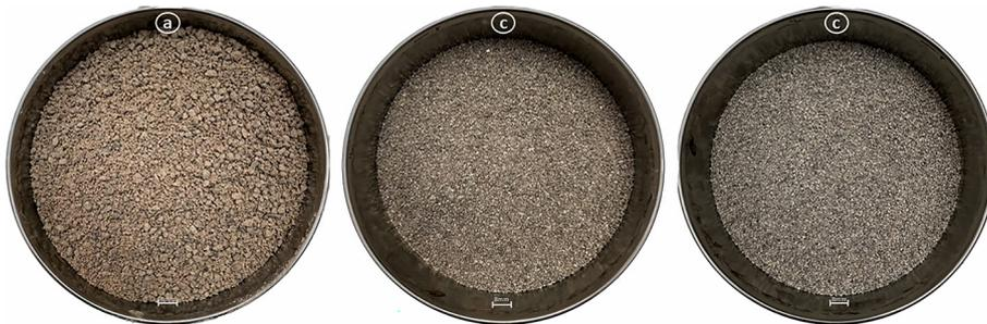
Figure 3. Varieties of sands employed in mortar mixtures; (a) raw natural sand, (b) washed natural sand, (c) recycled concrete sand
