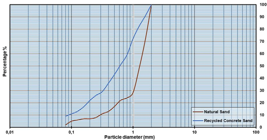
Figure 9. Particle size distribution of natural sand and recycled concrete sand
