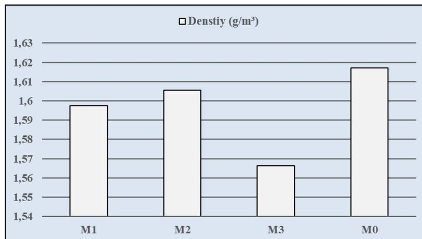
Figure 14. Density results of mortar mixes at different ages
