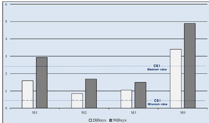
Figure 11. Compressive strengths of mortar mixes at different ages
