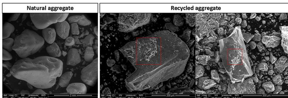
Figure 10. SEM images of aggregate at low magnification
