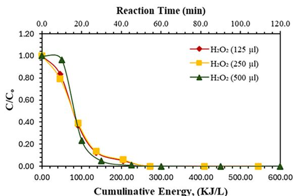
**Figure 2.** Photodegradation of ritonavir in Milli-Q assisted with H<sub>2</sub>O<sub>2</sub>
