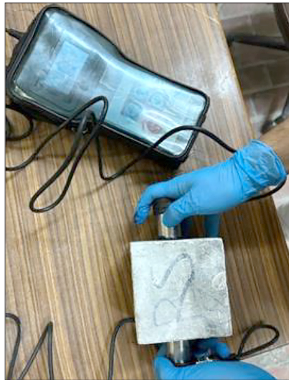
Figure 4. Ultrasonic pulse velocity test
