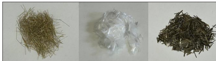
Figure 1. Fibers: (a) micro steel fiber, (b) polypropylene fiber, (c) basalt fiber
