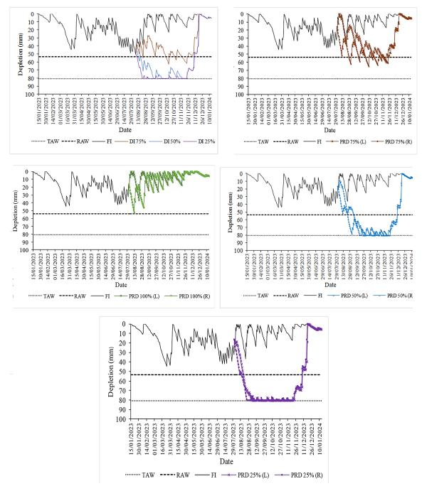
Figure 2. Daily patterns of soil water depletion (mm) in the root zone under full irrigation (FI), deficit irrigation with 75%, 50% and 25%ETc (DI-75%, DI-50%, DI-25%), and partial root-zone drying with 25%, 50% and 75% ETc (PRD-75%, PRD-50%, PRD-25%) alternating at 10 days, treatments. TAW: total available water, RAW: readily available water
