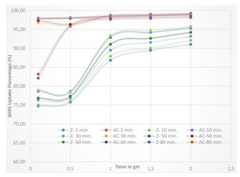
Figure 2. The uptake percentage of SDBS at different adsorbent doses of 0.1 g, 0.5 g, 1.0 g, 1.5 g, and 2.0 g
