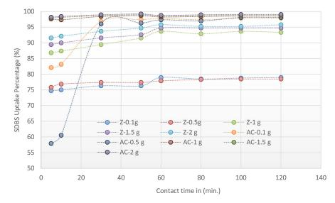
Figure 1. The percentage uptake of SDBS as function of time (5, 30, 50, 60, 80, 100, and 120 minutes) at different adsorbent doses of 0.1 g, 0.5 g, 1.0 g, 1.5 g, and 2.0 g
