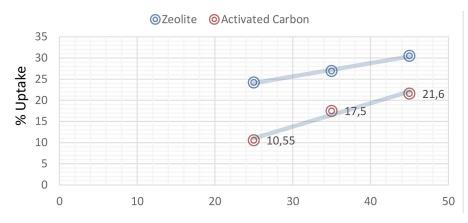
Figure 3. The percentage uptake of SDBS as a function of temperature (25, 35, 45 °C)
