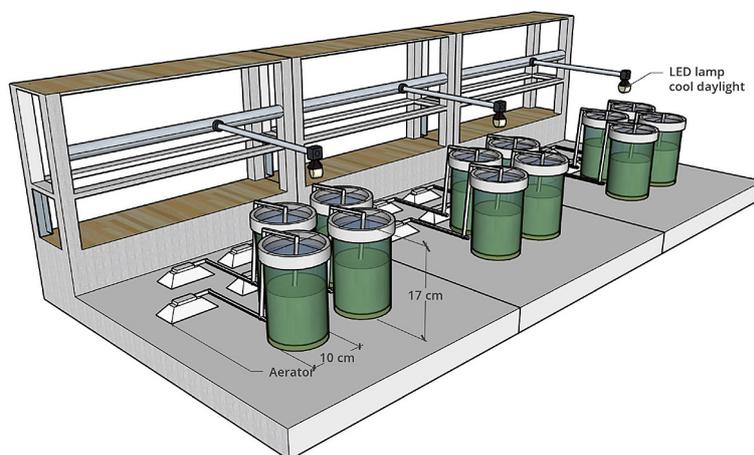
Figure 1. Design photobioreactor for the observation
