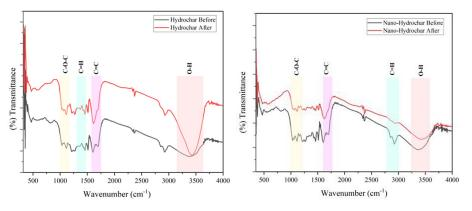
Figure 8. FTIR Spectrum of hydrochar and nano-hydrochar before and after adsorption
