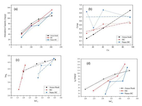
Figure 7. Consentration dan adsorption capasity plots of congo red adsorption (a) Langmuir isotherm, (b) Freundlich isotherm (c) and Temkin isotherm
