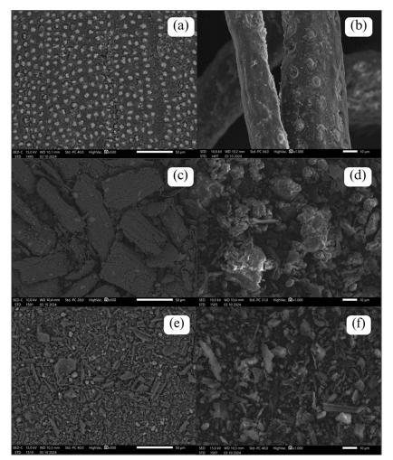
Figure 3. SEM image of Areca husk x500 (a), Areca husk x1000 (b), HC x500 (c), HC x1000 (d), nano HC x500 (e) and nano HC x1000 (f)
