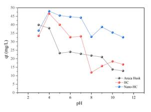
Figure 5. Impact of pH adsorption to Areca husk, hydrochar and nano-hydrochar
