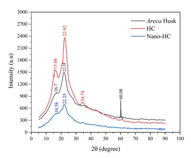
Figure 1. X-ray diffraction of Areca husk, HC and nano HC
