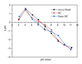
Figure 4. pHpzc point zero charge of Areca husk, HC and nano HC
