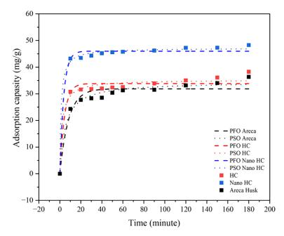
Figure 6. Adsorption kinetics pseudo-first order kinetic model and pseudo-second order kinetic model of Areca husk, HC and nano HC
