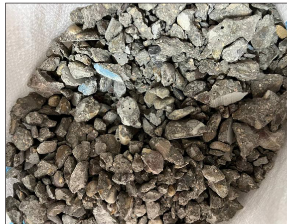
Figure 4. RCA-made of crushing concrete
