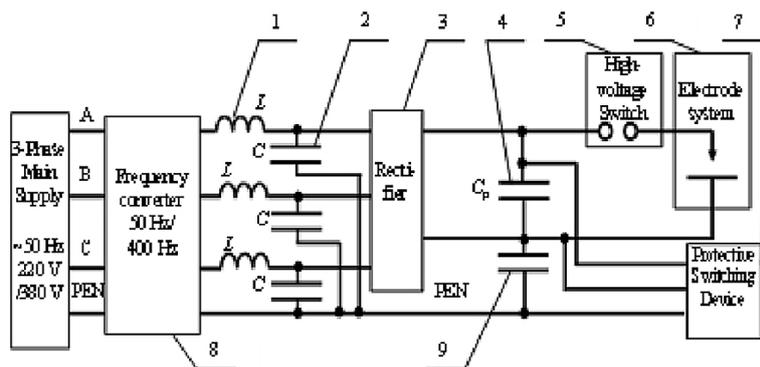
Figure 1. Laboratory electric discharge installation (Vinnychenko et al., 2024)
