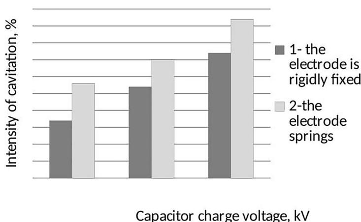
**Figure 3.** The influence of the electrode system design on the intensity of electric discharge cavitation
