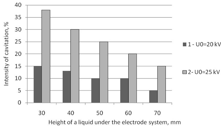
**Figure 4.** Dependence of the intensity of electric discharge cavitation on the level of the working fluid above the electrode system
