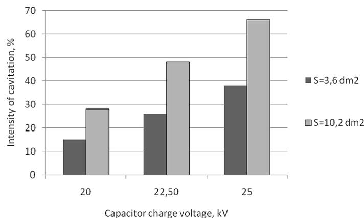
**Figure 5.** Dependence of the intensity of electric discharge cavitation on the surface area of the liquid in the working chamber
