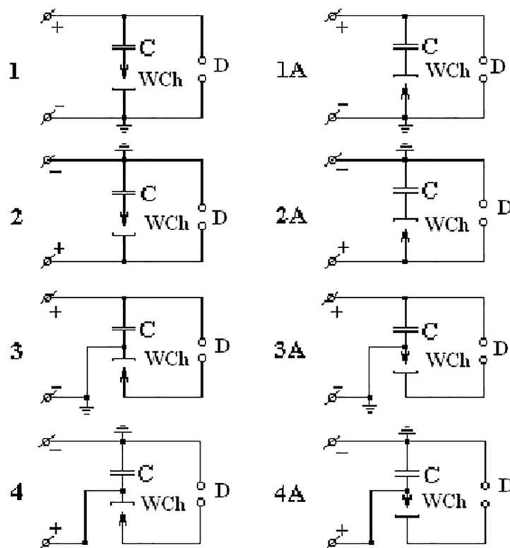
**Figure 2.** Energy storage device (capacitor bank) charging schemes: *C* – battery of capacitors, *D* – discharger, *WCh* – working chamber
