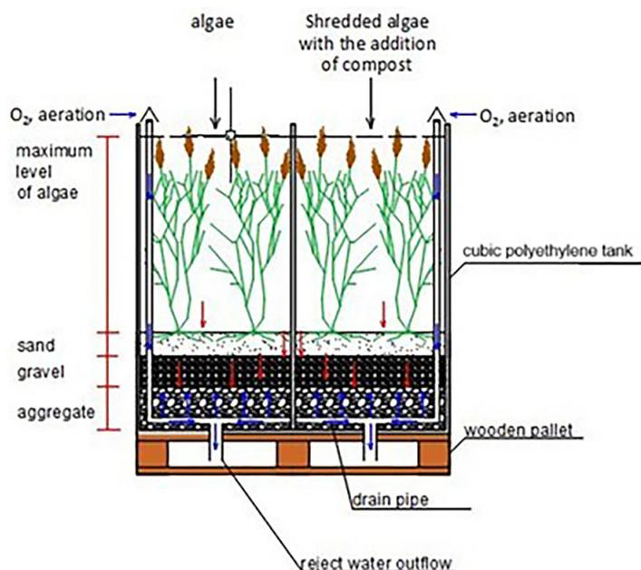
Figure 1. Scheme of one module cube of pilot RBS (Kupczyk's study)
