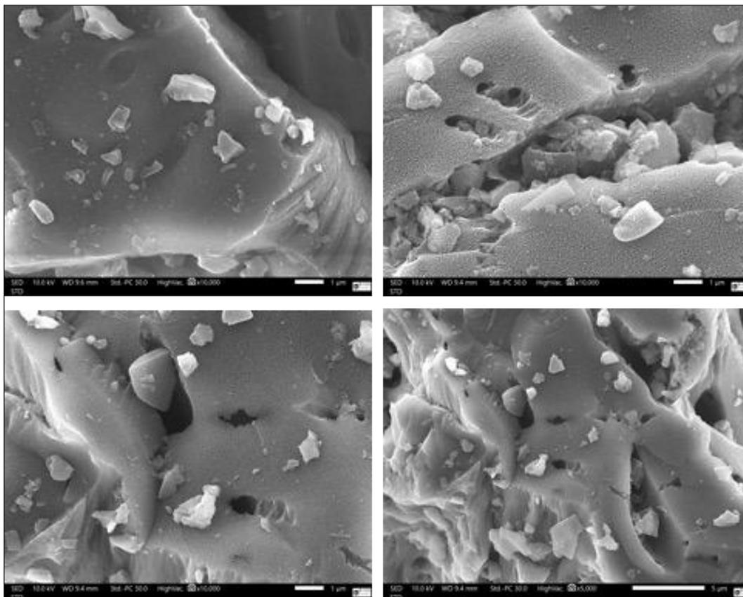
Figure 7. SEM of biochar after activation
