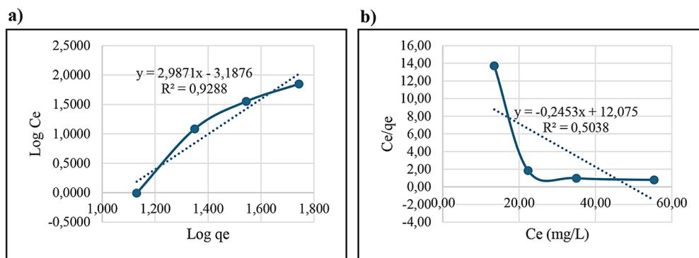
Figure 5. Isotherm analysis for phosphate adsorption: (a) Isotherm Freundlich (b) Isotherm Langmuir
