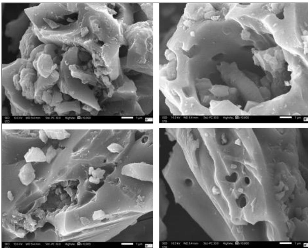
**Figure 6.** SEM of biochar before activation
