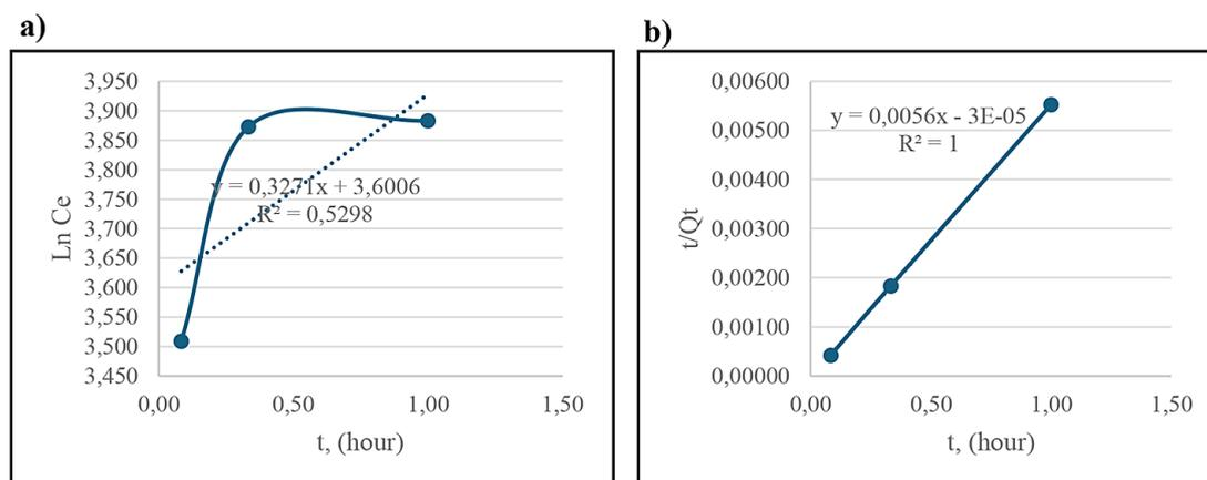
**Figure 2.** Kinetic reaction first order (a) and second order (b) for ammonium adsorption
