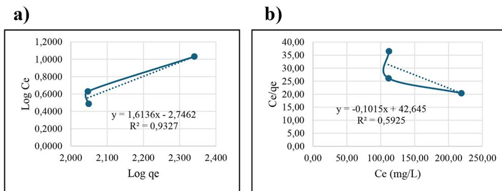
Figure 4. Isotherm analysis for ammonium adsorption: (a) Isotherm Freundlich (b) Isotherm Langmuir
