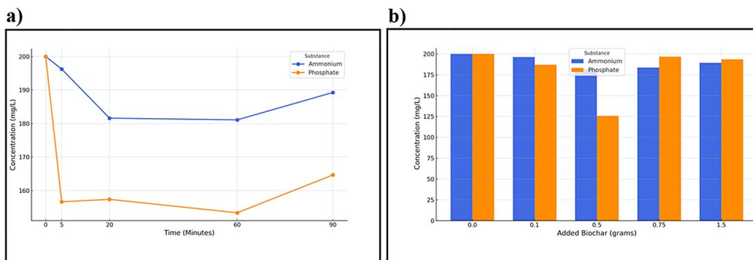
**Figure 1.** The nutrient concentration during the adsorption according to contacted time (a) and added biochar (b)
