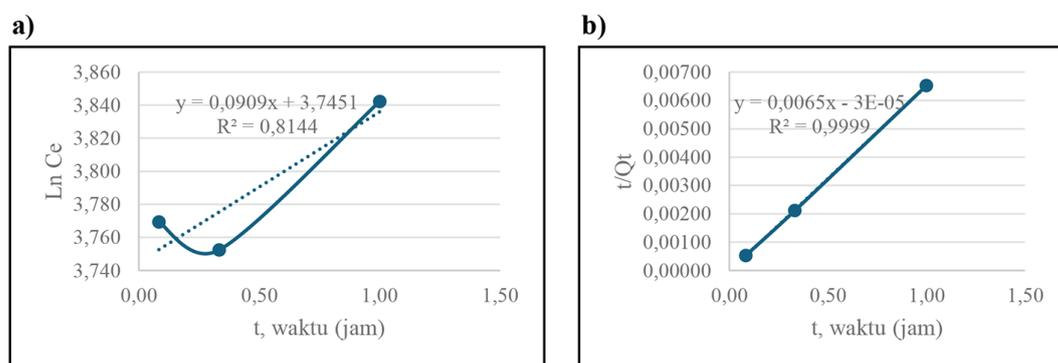
**Figure 3.** Kinetic reaction first order (a) and second order (b) for phosphate adsorption
