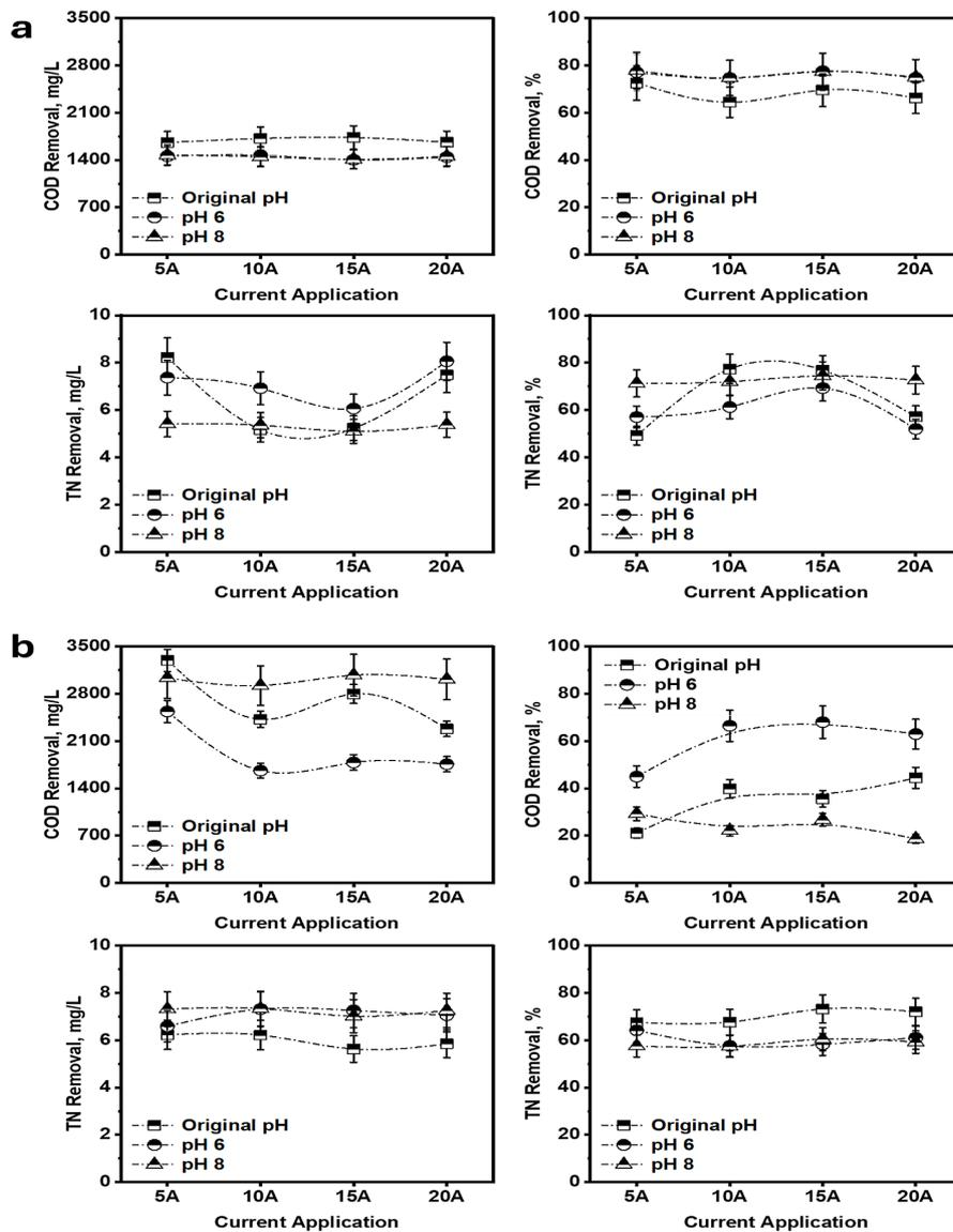
Figure 5. TN and COD removal during electrocoagulation processes; (a) Fe electrodes and (b) Al electrodes with the pH differential
