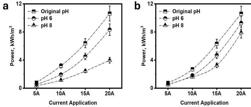
Figure 3. Power consumption during electrocoagulation (a) Al and (b) Fe electrode
