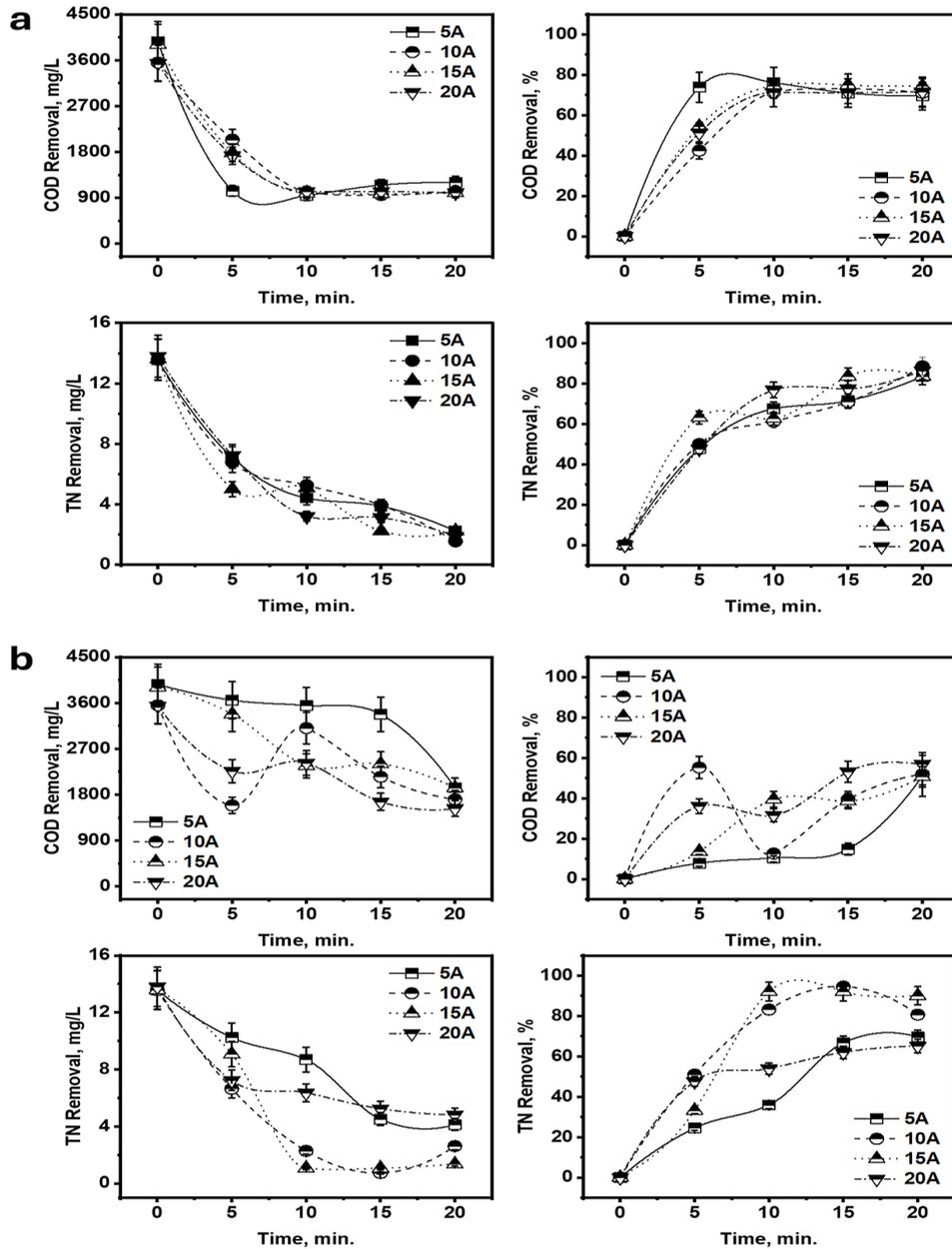
**Figure 2.** COD and TN removal using (a) Fe and (b) Al electrode with the current application strategy and pH differential
