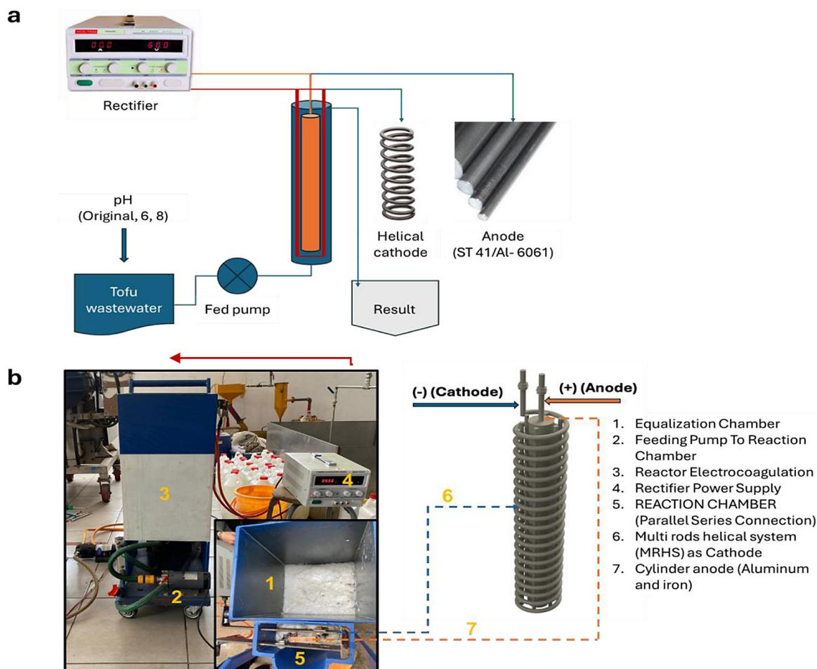
**Figure 1.** (a) Configuration of the electrocoagulation-based tubular system; and (b) a pilot scale visualization of the electrocoagulation reactor in this study using an MRHS in continuous flow
