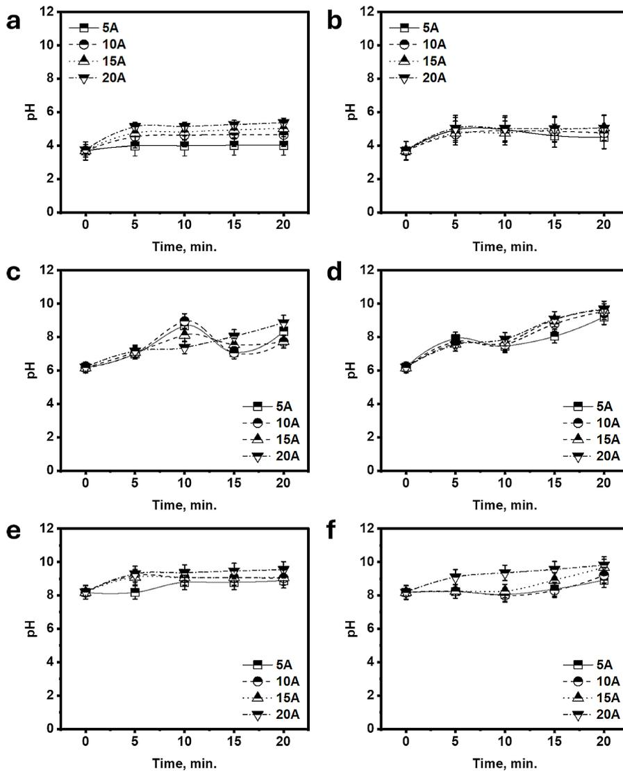
Figure 4. pH during electrocoagulation processes; (a, b, c) Al electrodes; (d, e, f) Fe electrodes
