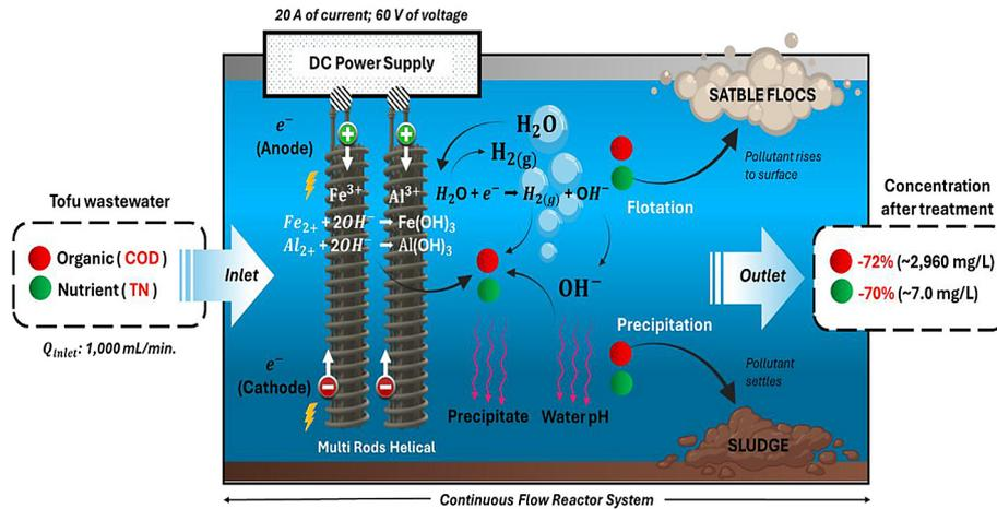
Figure 6. COD and TN removal in EC based continuous flow reactor system using a MRHS cathode and Fe/Al anode
