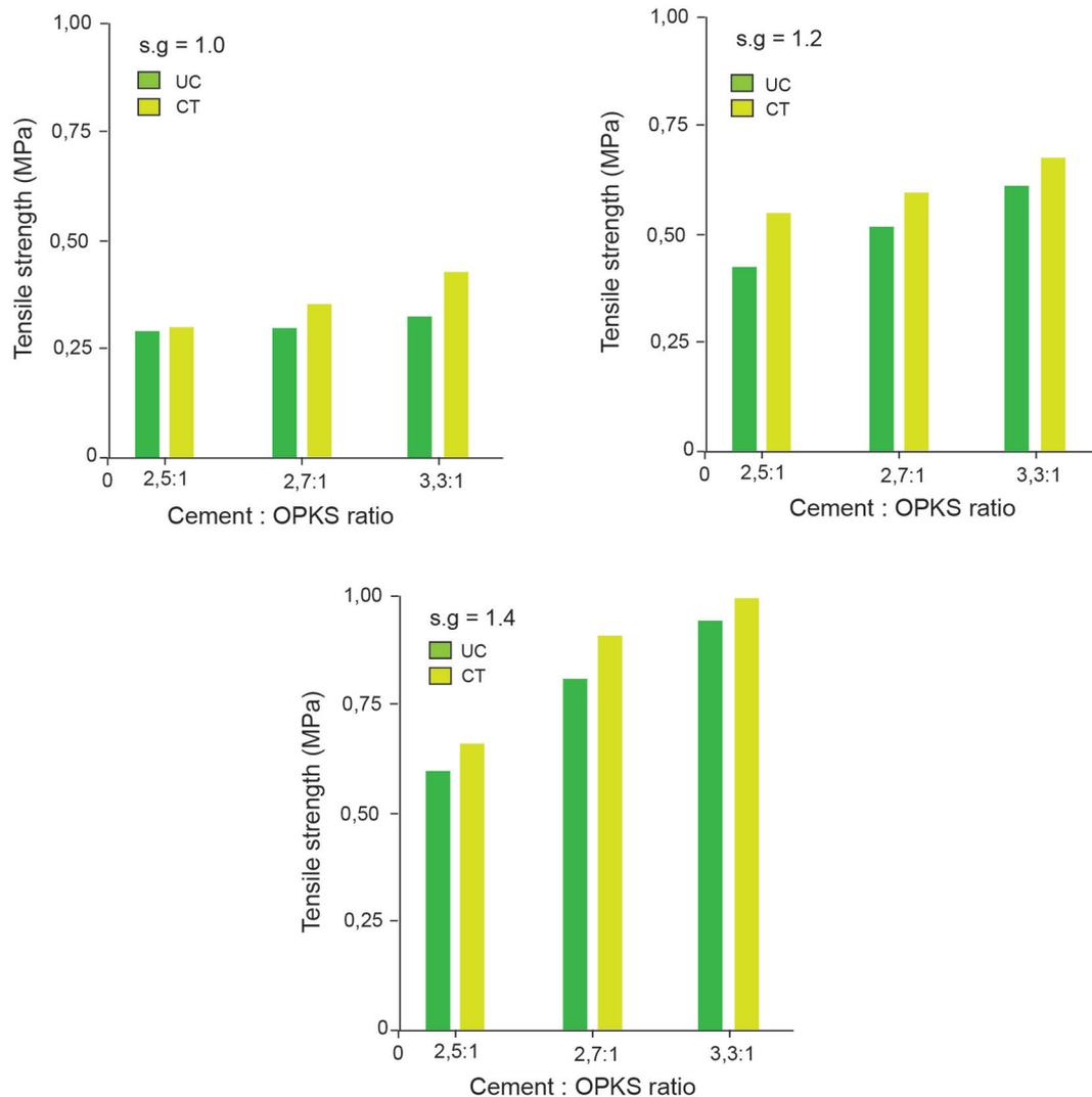
**Figure 5.** Tensile strength development of OPKS-based LWFC over 28-day curing period at s.g. of 1.0, 1.2, and 1.4: comparison between UC and CT at varying cement-to-OPKS ratios
