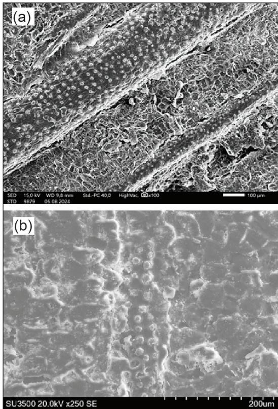
**Figure 2.** Surface characterization of OPKS using SEM: (a) uncoated and (b) silane-siloxane (5%) coated specimens at 200 μm magnification
