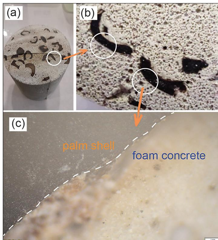
**Figure 3.** Optical microscopy characterization: (a) internal structure of LWFC, (b) embedded OPKS aggregate morphology, and (c) interface bonding at the OPKS-cement matrix boundary zone
