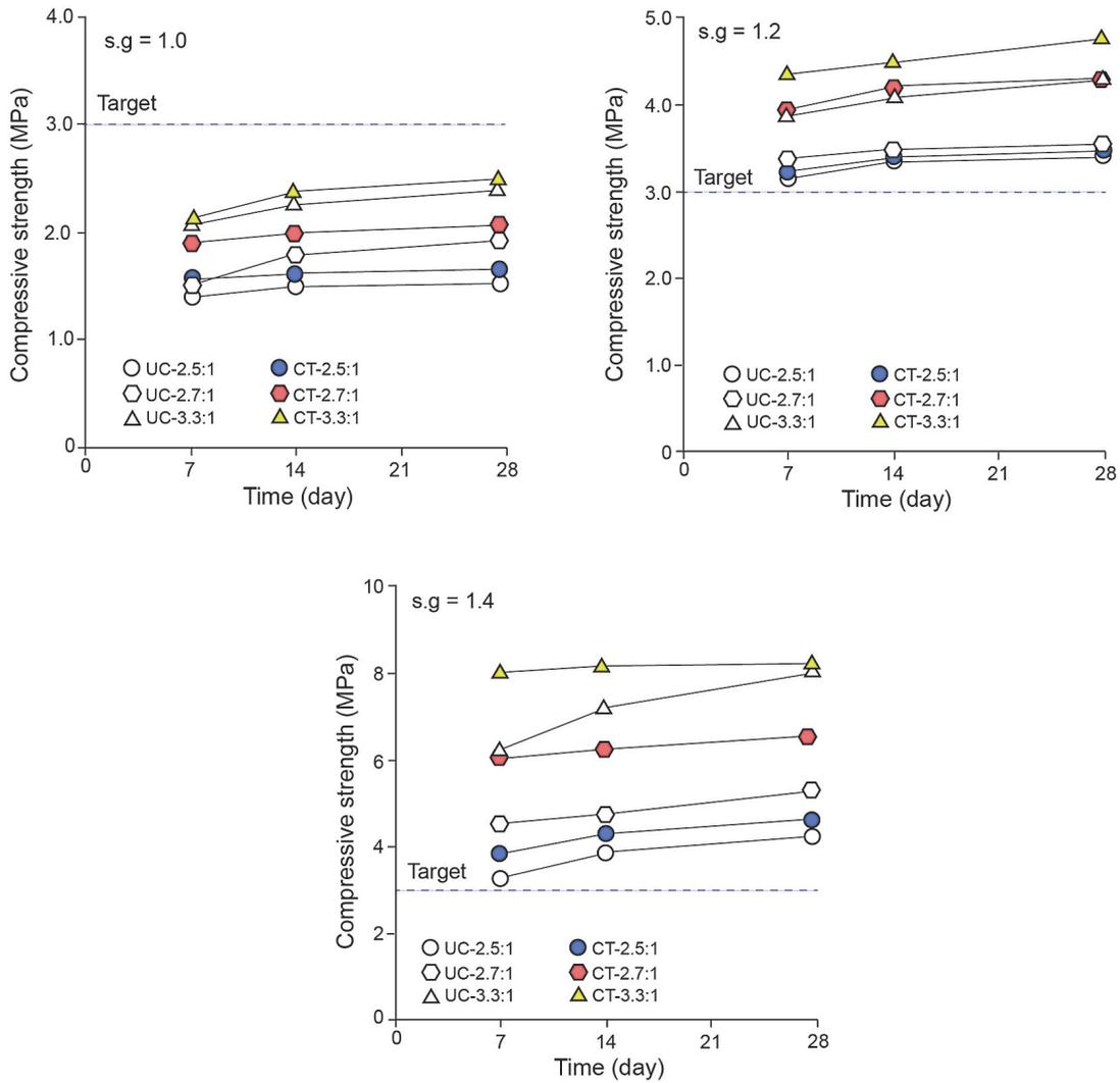
**Figure 4.** Compressive strength development of OPKS-based LWFC over 28-day curing period at s.g. of 1.0, 1.2, and 1.4: comparison between UC and CT at varying cement-to-OPKS ratios
