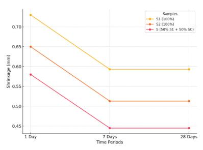
Figure 9. Shrinkage variation over time (1 day, 7 days, and 28 days) for three different samples
