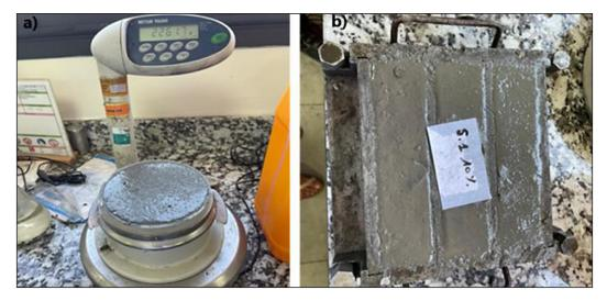
Figure 6. Density measurement (a), and filling of the mini cone using the MBE (b)
