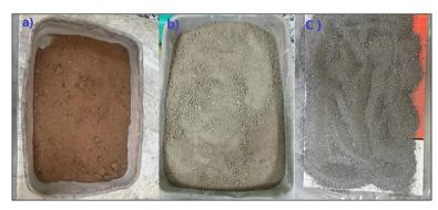
Figure 3. Dune sand (a), dredged sediments (b), and crushed sand (c) used for the formulations
