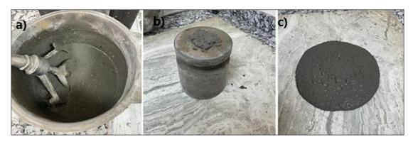
Figure 5. Mixing of concrete in the mixing container (a), filled cylindrical mold for slump flow test (b), spread of concrete after the slump flow test (c)
