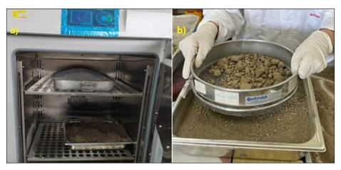
Figure 4. Samples dried at 105 °C (a), and sieved through 4 mm mesh sieves (b)
